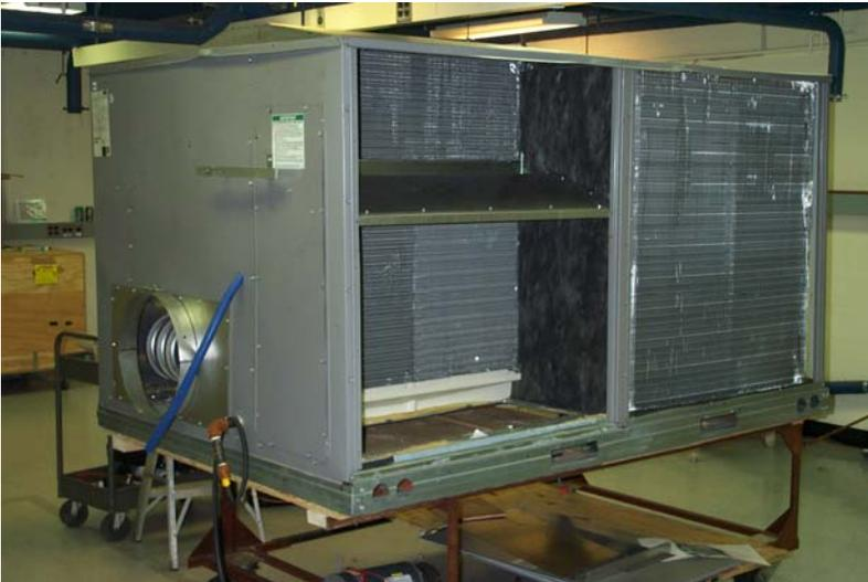
**Figure 18: Completed IDOAS Prototype**
