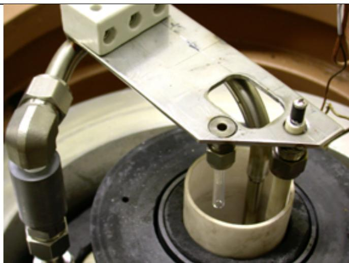
**Figure 4.4 Second generation of feedthrus on elevator**
