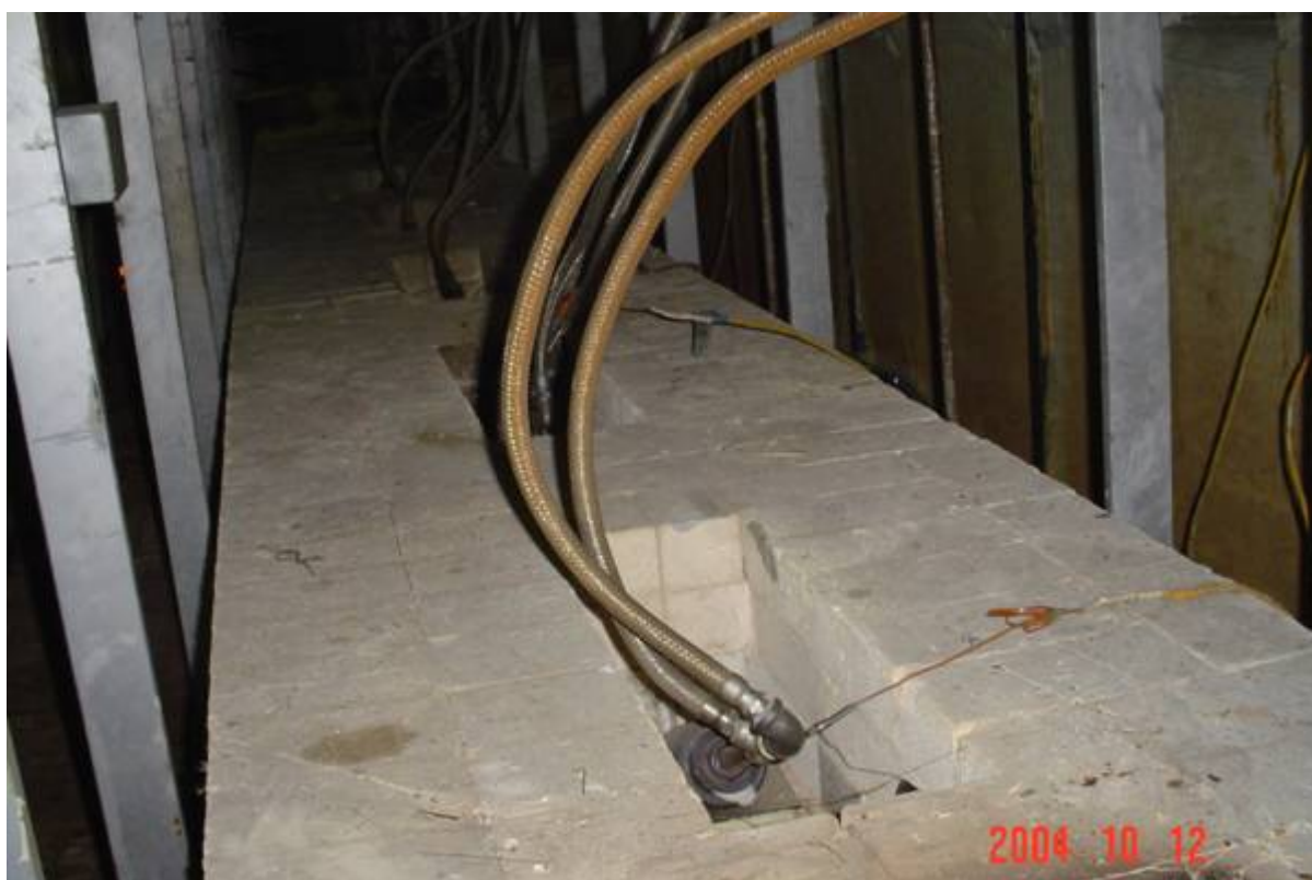
Fig. 10 Front End Oxy-Fuel burner in operation in Owens Corning's Jackson TN plant
