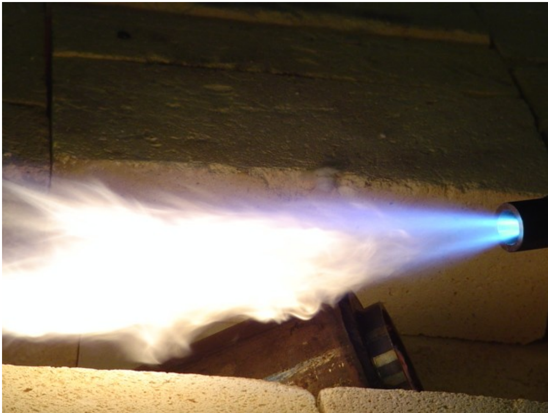
Fig. 7 Flame of Venturi style burner
