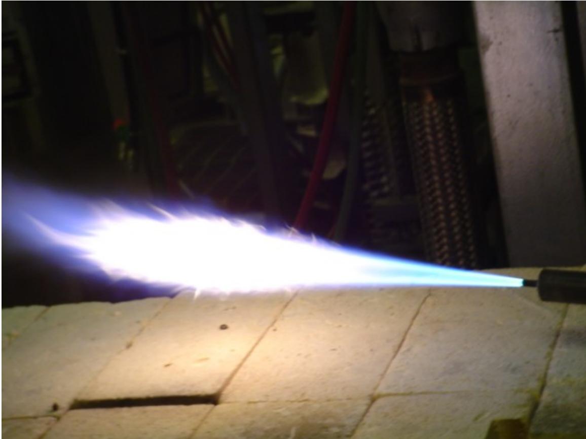
Fig. 8 Flame of Basic OC design burner
