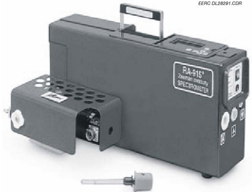
Figure 4. Ohio Lumex instrument (Lumex-915+ with RP-M 324 attachment).
