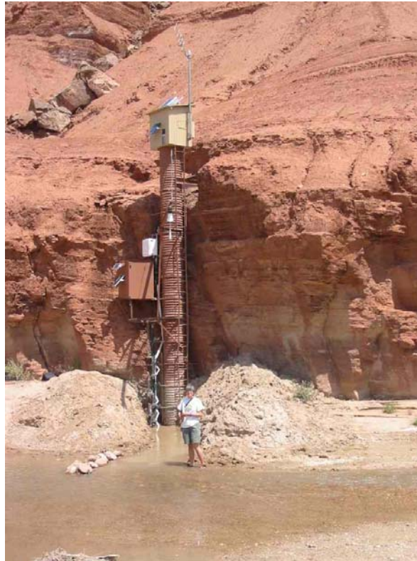
Figure 5.1: View of the USGS gauging station at the Paria. The TDR monitoring system is mounted on the frame work of the USGS station and consists of the white enclosure seen midway up the stilling station above the larger brown enclosure and a stack of TDR probes immediately to the left of the stilling station. See Figure 4.2 for a close-up view of the TDR stack.
