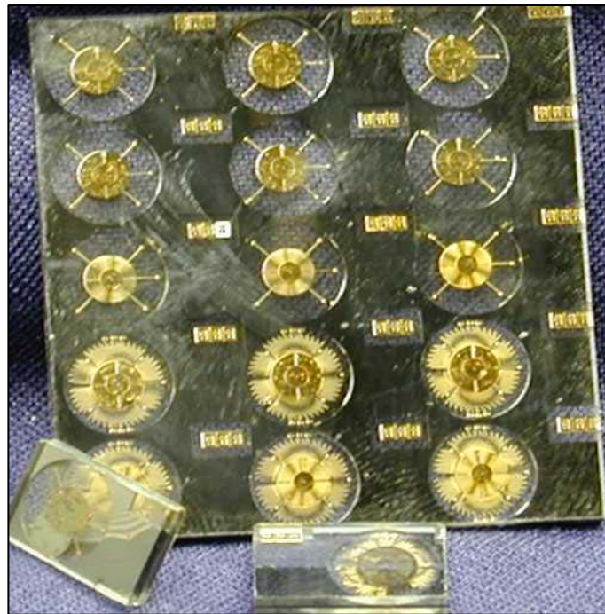
Figure 9: Wafer-Level Batch Processing of Stators Enables Low Cost
