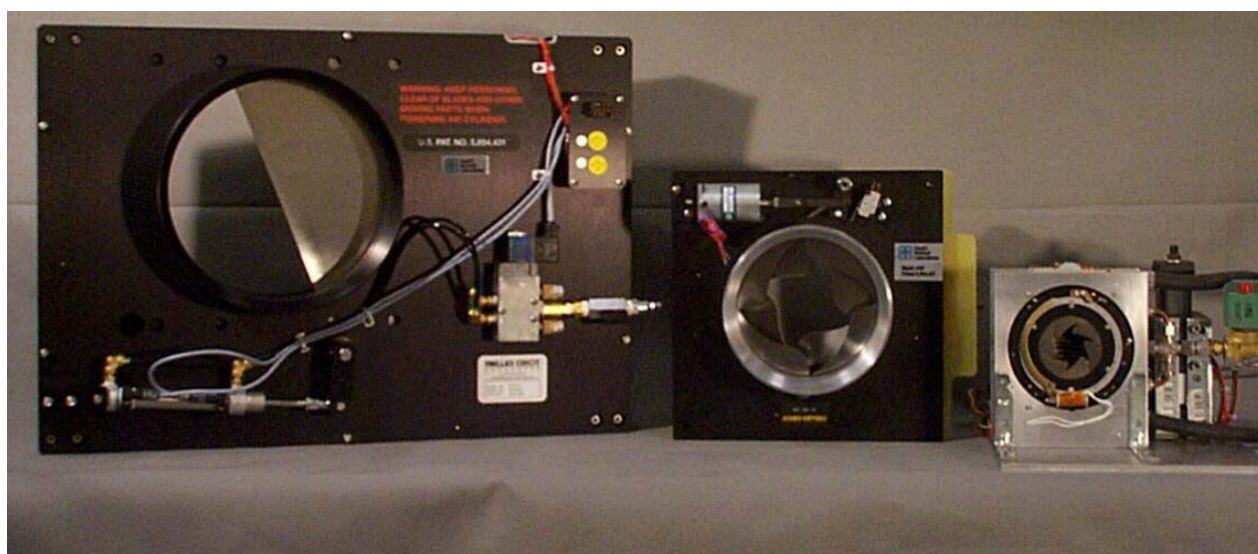
Figure 10. Sandia Large-Volume Preconcentrators (Inlet sizes: 9-inch, 6-inch, 2-inch)
