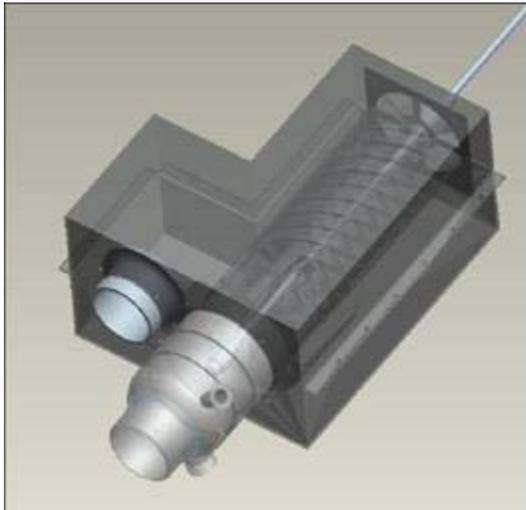
Figure 5: APH metallic hybrid using a 6 fin ceramic heat exchanger element
