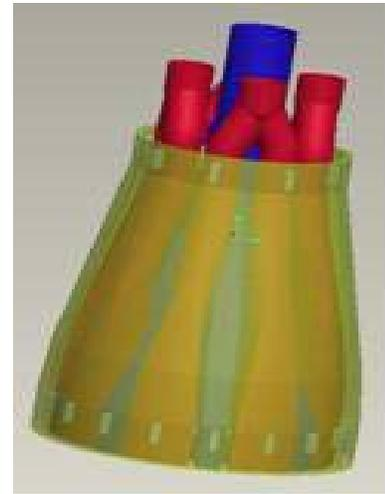
Figure 2: Three-powder heat exchanger forming tool
