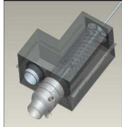
Figure 9: Metallic Hybrid APH system utilizing an integral ceramic heat exchanger and burner.
