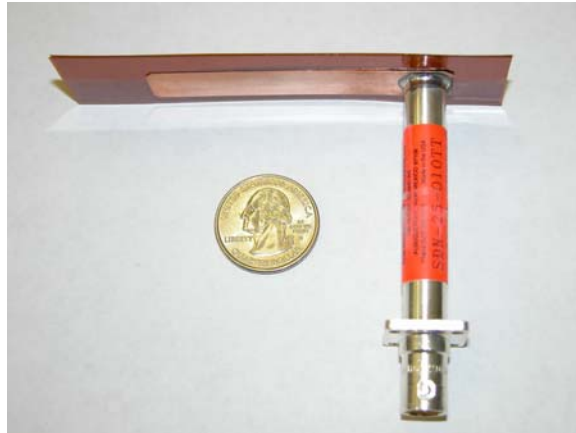
Figure 4: Current Viewing Resistor
