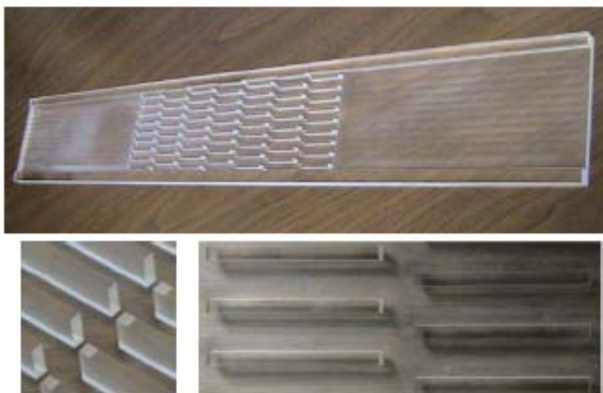
Figure 10. Acrylic test section fin part of 1:3 dimension ratio.
