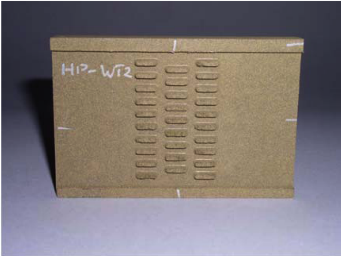
Figure 7. DLR prototype wood composite test plate (80x120mm) with fins (~10mm).
