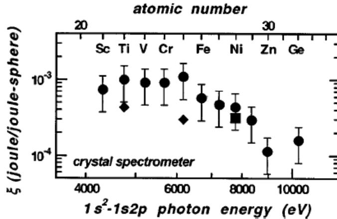
FIG. 5. Conversion efficiency (circles) measured with the convex crystal spectrometer for the He-like  $1s^2-1s2p_{,s}$  group of lines compared to Philion *et al.* for 550 ps (square) and 125 ps (diamonds) laser pulses.
