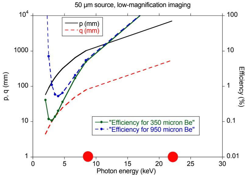
Figure 9: Required full-source imaging parameters to match Kevex resolution, contrast, and signal-to-noise, with a 50  $\mu\text{m}$  source and low magnification. Required efficiencies assume a 300-J laser and 50% detection efficiency. Also plotted are experimental data points from Titan area backlight targets.
