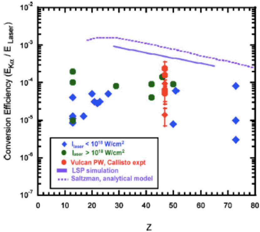
FIG. 5. (Color online)  $K\alpha$  conversion efficiency as function of target  $Z$  including other experiments (see the text). The diamond plotting symbols correspond to data with  $I_L < 10^{18}$  W/cm<sup>2</sup> and the circles to  $I_L > 10^{18}$  W/cm<sup>2</sup>. The solid line represents the prediction from the LSP modeling and the dotted line is analytical model prediction from Saltzman.
