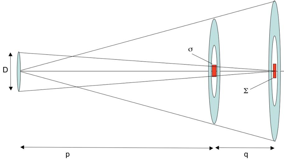
Figure 3(b): Full-source radiography.  $D$  is the x-ray source diameter,  $p$  is the distance between the source and the object,  $q$  is the distance between the object and the detector,  $\sigma$  is the resolution at the object, and  $\Sigma$  is magnified resolution at the detector plane. The sketch illustrates a low-magnification geometry, but high magnification could be used as well if the source size is small enough, as shown in Fig. 1.
