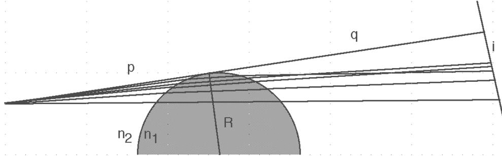
Figure 2: Sketch of ray paths for imaging the limb of a DT layered capsule.  $p$  is the source/object distance,  $q$  is the object/detector distance,  $n_2$  is the refractive index of the ice,  $n_1 > n_2$  is the refractive index of the central gas,  $R$  is the inner ice surface radius, and  $i$  is the width of the projected phase-contrast dark band.
