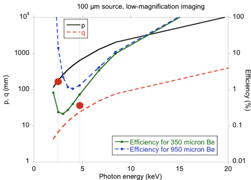
Figure 5: Required full-source imaging parameters to match Kevex resolution, contrast, and signal-to-noise, with a 100  $\mu\text{m}$  source and low magnification. Required efficiencies assume a 600-J laser and 50% detection efficiency. Also plotted are experimental data from Janus.
