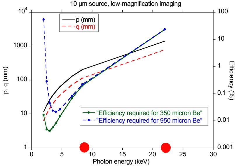
Figure 10: Required full-source imaging parameters to match Kevex resolution, contrast, and signal-to-noise, with a 10  $\mu\text{m}$  source and low magnification. Required efficiencies assume a 300-J laser and 50% detection efficiency. Also plotted are experimental data points from Titan restricted source targets.
