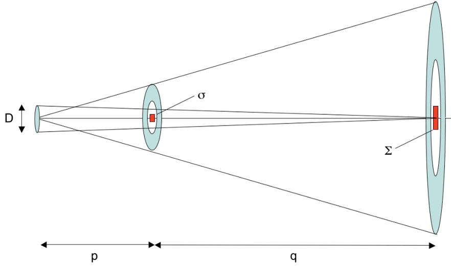
Figure 1: High-magnification radiography with a small source.  $D$  is the x-ray source diameter,  $p$  is the distance between the source and the object,  $q$  is the distance between the object and the detector,  $\sigma$  is the resolution at the object, and  $\Sigma$  is magnified resolution at the detector plane.
