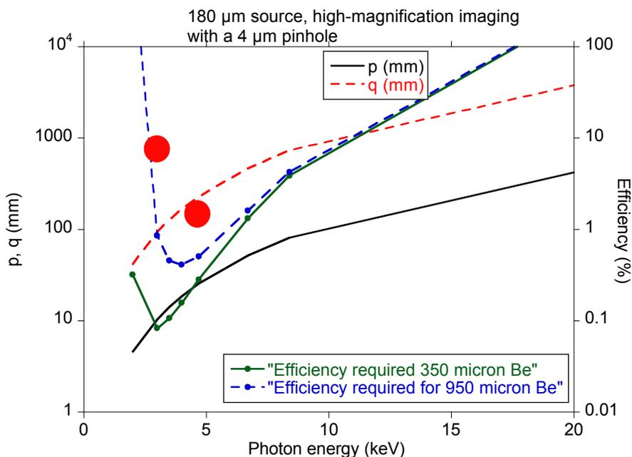
Figure 12: Required pinhole-restricted high-magnification imaging parameters to match KeveX resolution, contrast, and signal-to-noise, with a 180  $\mu\text{m}$  source and a 4  $\mu\text{m}$  pinhole. Required efficiencies assume a 5 kJ 2-ns laser and 50% detection efficiency. Also plotted are expected efficiencies for optimized 351-nm sources at  $1\text{e}16 \text{ W}/\text{cm}^2$ .
