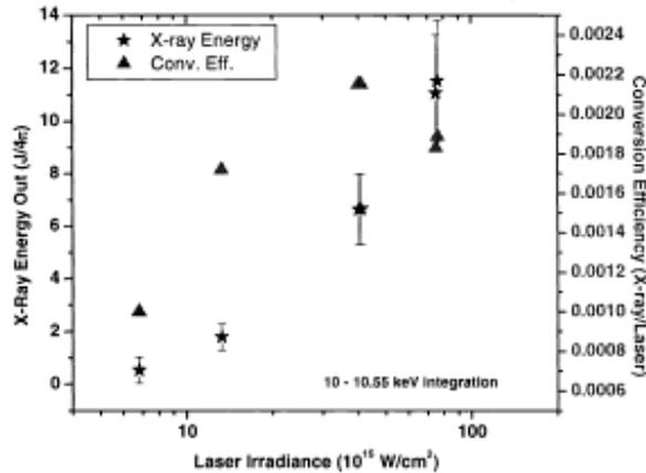
Figure 5: Scaling of Ge emission and conversion efficiency at 10.3 keV as a function of laser irradiance. All shots were taken at best focus ( $\sim 100\mu\text{m}$ ) using one, two, six and 12 beams respectively. At 6 and 12 beams there are duplicate data sets.
