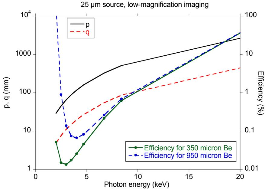
Figure 4(a): Required full-source imaging parameters to match Kevex resolution, contrast, and signal-to-noise, with a 25  $\mu\text{m}$  source and low magnification. Required efficiencies assume a 600-J laser and 50% detection efficiency.
