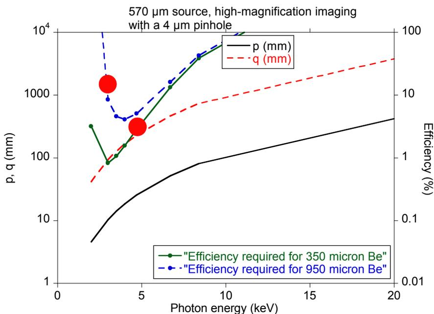
Figure 11: Required pinhole-restricted high-magnification imaging parameters to match KeveX resolution, contrast, and signal-to-noise, with a 570  $\mu\text{m}$  source and a 4  $\mu\text{m}$  pinhole. Required efficiencies assume a 5 kJ 2-ns laser and 50% detection efficiency. Also plotted are expected efficiencies for optimized 351-nm sources at  $1\text{e}15 \text{ W}/\text{cm}^2$ .
