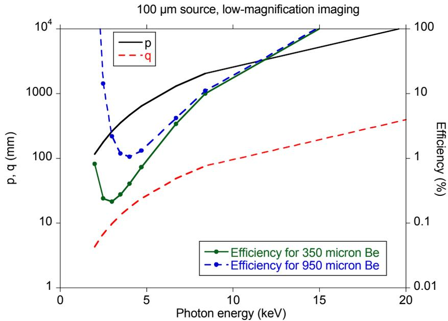
Figure 4(b): Required full-source imaging parameters to match Kevex resolution, contrast, and signal-to-noise, with a 100  $\mu\text{m}$  source and low magnification. Required efficiencies assume a 600-J laser and 50% detection efficiency.
