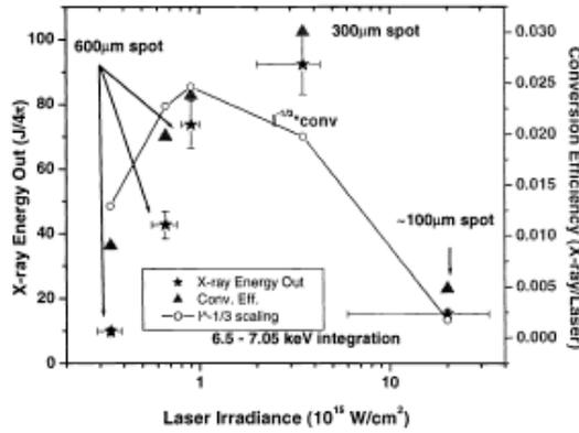
Figure 3: X-ray yield scaling and conversion efficiency from Fe targets as a function of laser irradiance. The left vertical axis is the energy generated at the source into  $4\pi$  steradians without correction for crystal reflectivity. The right vertical axis is the conversion of laser energy into x-ray energy. The additional curve is a power law for the irradiance,  $I^{-1/3}$ , which is typically used for conversion efficiency.
