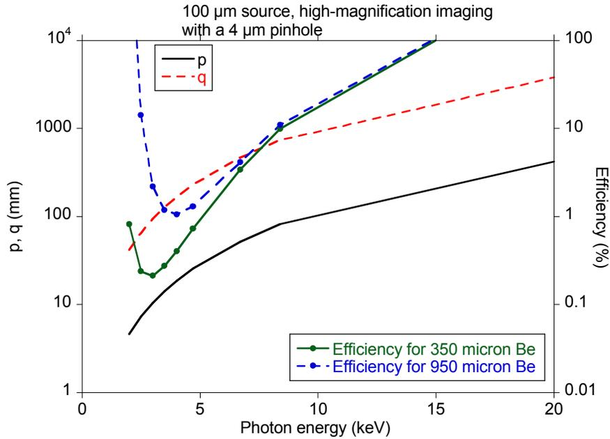
Figure 4(d): Required pinhole-restricted high-magnification imaging parameters to match Kevex resolution, contrast, and signal-to-noise, with a 100  $\mu\text{m}$  source and a 4  $\mu\text{m}$  pinhole. Required efficiencies assume a 600-J laser and 50% detection efficiency.
