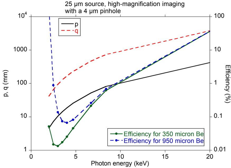
Figure 4(c): Required pinhole-restricted high-magnification imaging parameters to match Kevex resolution, contrast, and signal-to-noise, with a 25  $\mu\text{m}$  source and a 4  $\mu\text{m}$  pinhole. Required efficiencies assume a 600-J laser and 50% detection efficiency.
