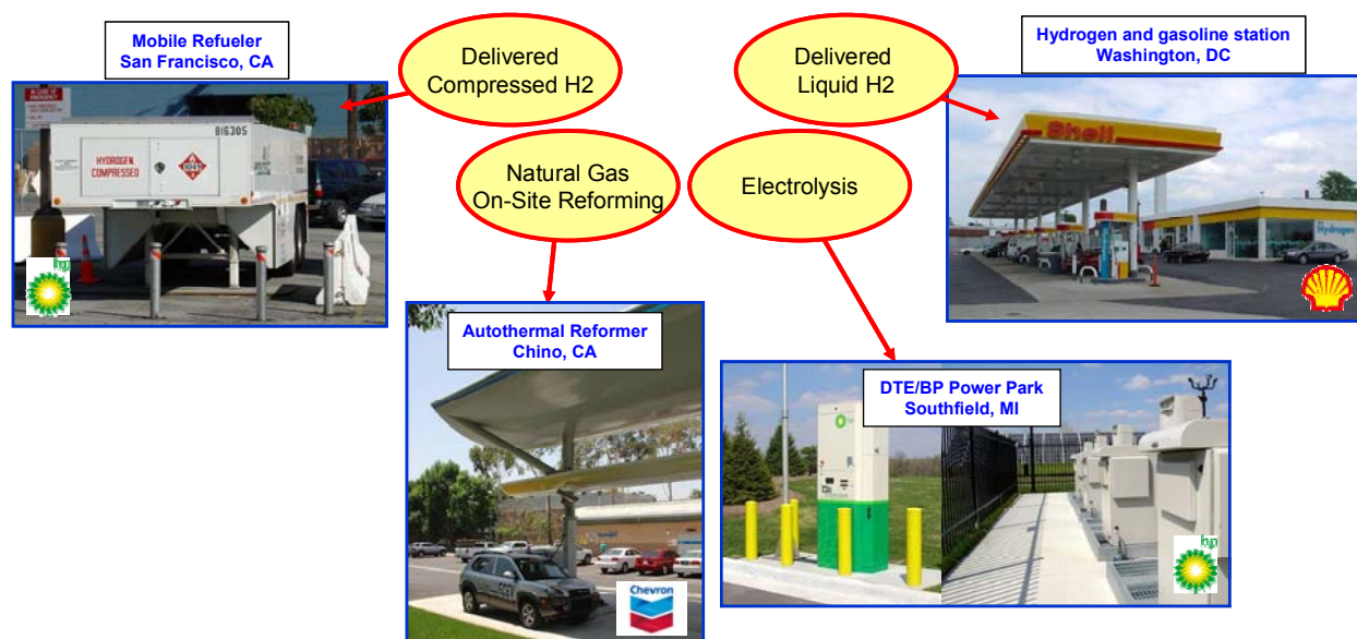
Figure 2: Four Types of Hydrogen Production and Refueling Facilities with Examples
