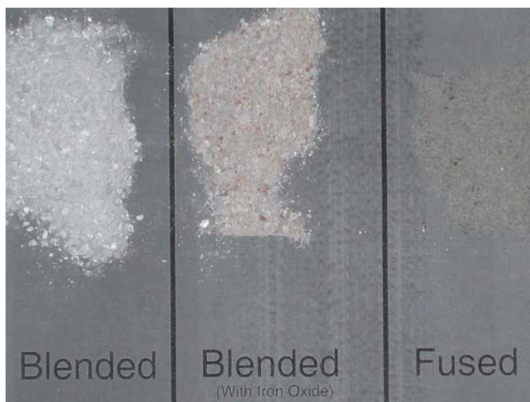
Figure 3: MgCl 2 - KCl salts in blended and fused forms
