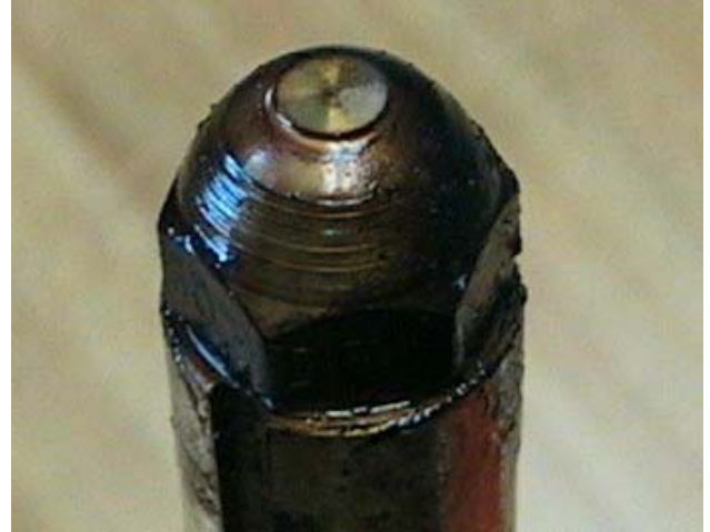
Figure 6 Nozzle after 4,650 hours
