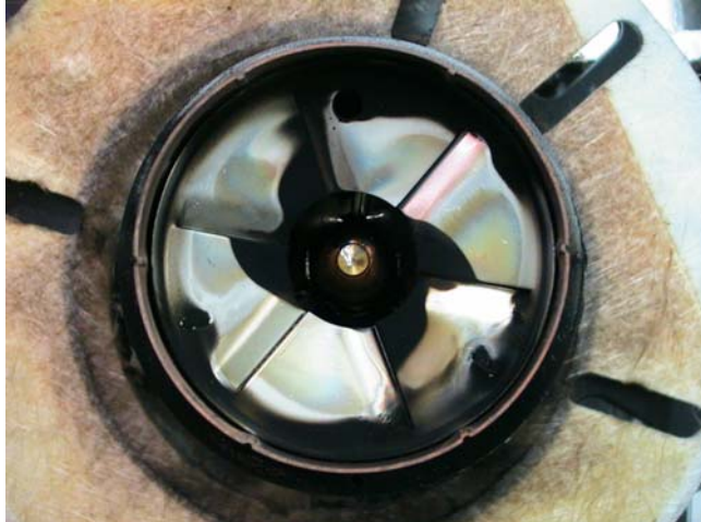
Figure 5 Combustion head and nozzle
