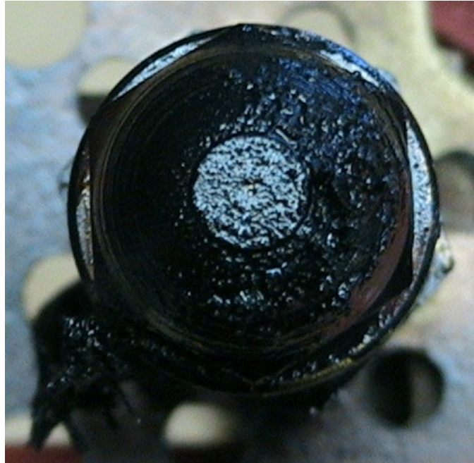
Figure 9 Fouled nozzle tip, after 1405 hours of on-time operation
