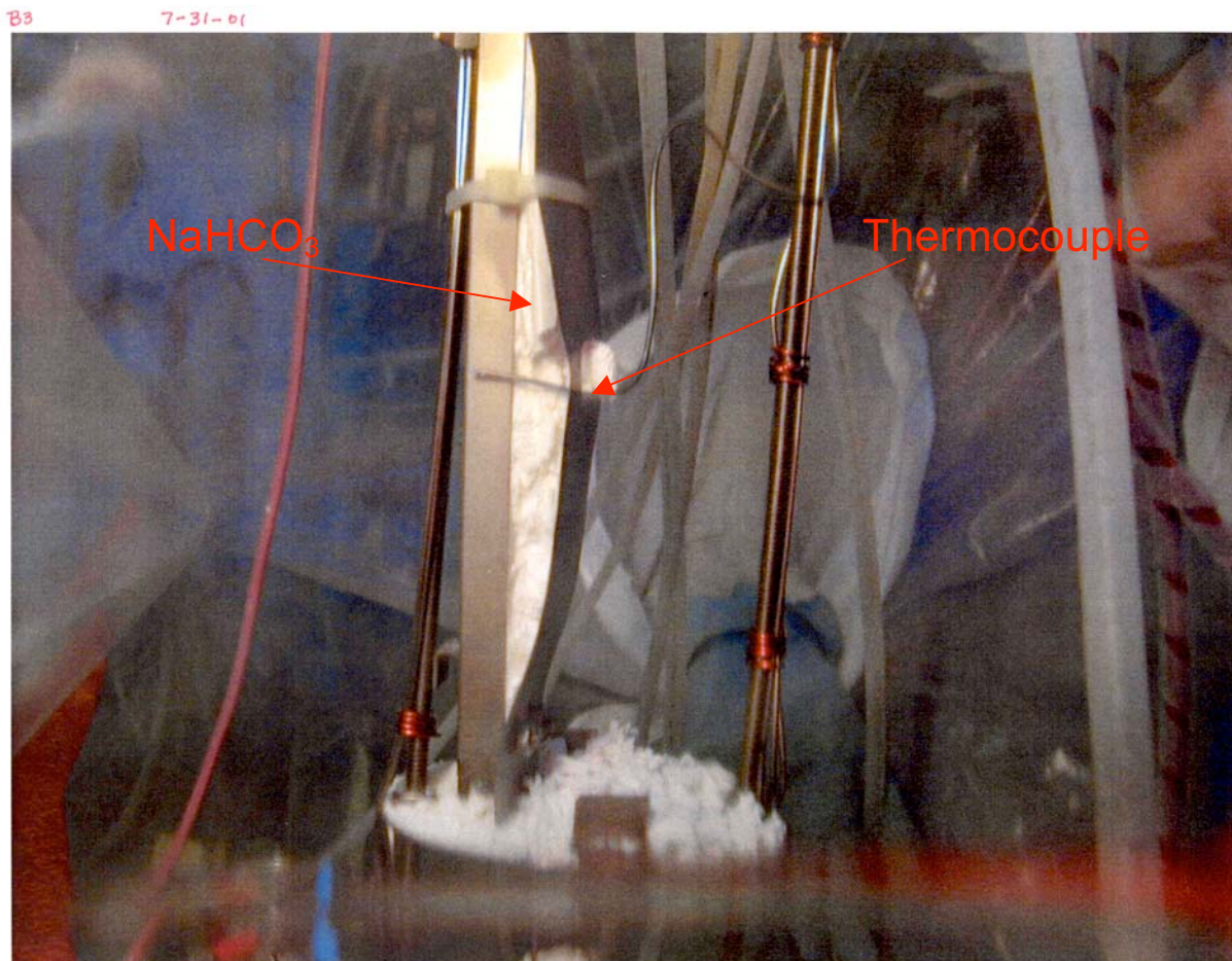
Figure 12. Tray B3 after 29 days of exposure (shown in vertical alignment). The wire in the center is a thermocouple.
