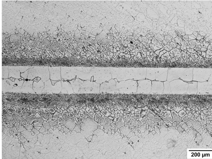
Figure 21. Etched metallographic cross-section of well-bonded area of braze joint.
