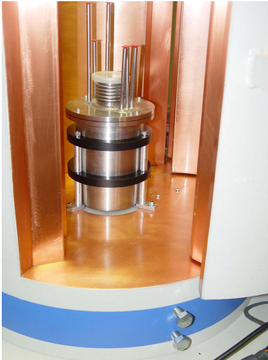
Figure A-4. The G4 spectrometer shield interior with a sample chamber similar (but not identical) to those to be used during AGR-1. This chamber has several flange penetrations that will not be in the AGR-1 design. The AGR-1 top flange will be penetrated only by a gas inlet tube and a gas outlet tube.
