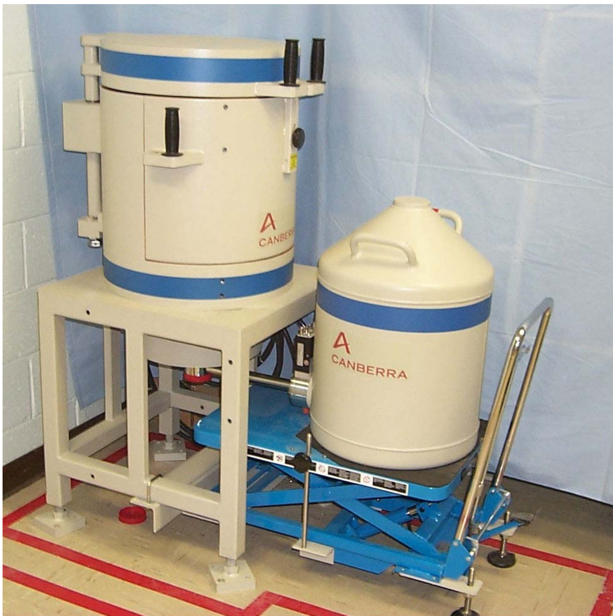
Figure A-1. Photograph of the assembled G3 spectrometer. The detector is raised into its measurement position.
