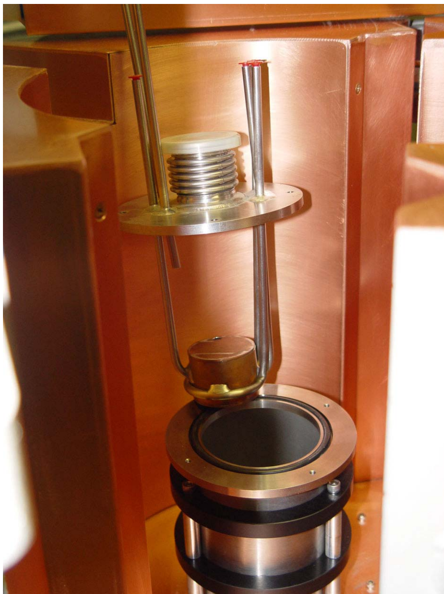
Figure A-5. Sample chamber interior view showing the flow-through 50 cm 3 sample volume normally contained in the outer containment “beaker”.
