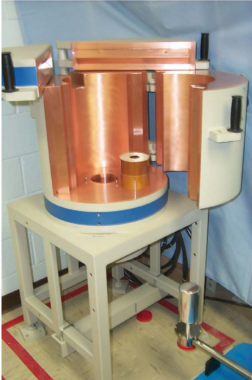
Figure A-2. G3 spectrometer with the front and top doors open, detector removed (detector head is visible extending in from bottom right), and the collimator removed from the bottom center of the shield floor.
