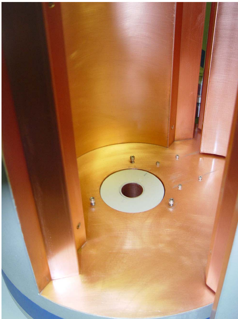
Figure A-3. Close up of the interior of the G4 spectrometer shield with the 32 mm collimator aperture in place. The detector face is positioned 127 mm below the interior face of the 114 mm thick collimator, thus is 13 mm (0.5 in) below the lower collimator face.
