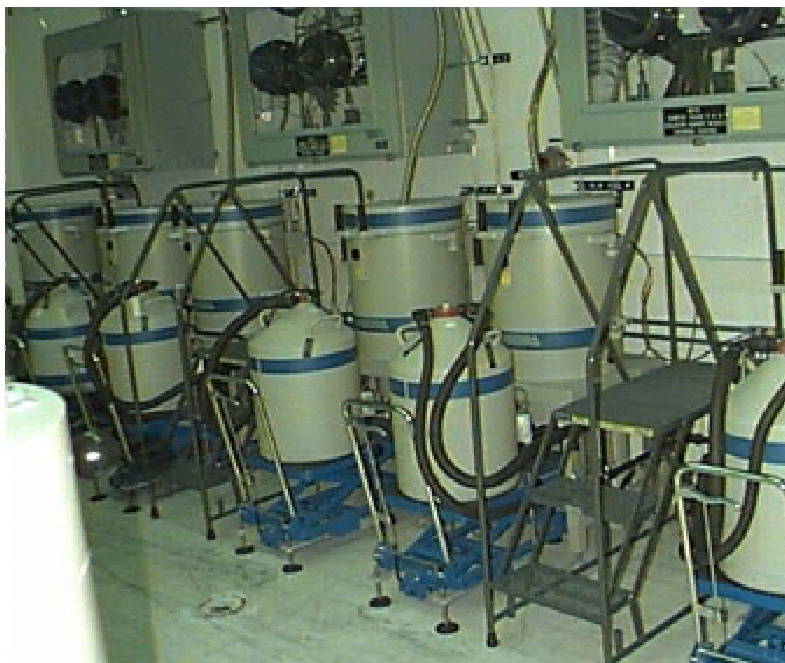
Figure 3. Six gamma-ray spectrometers presently installed in the ATR. These are similar to those planned for AGR-1.
