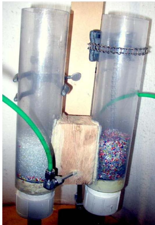
Figure 1. A cold flow model of a dual fluidized bed was produced to test transport of the fluidizing material between the two beds.
