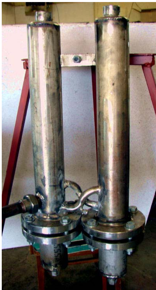
Figure 2. The stainless steel working dual fluidized bed prototype.
