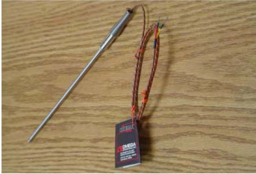
Figure 11 The Thermocouple Probe (K-Type) for Gasifier Simulator (Hot Model)
