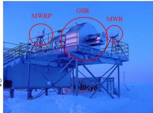
Figure 2. Photo of the deployments of the Microwave Profiler (MWRP), the Ground-based Scanning Radiometer (GSR), and the Microwave Radiometer (MWR) at the NSA/AAO during WAMOP04.
