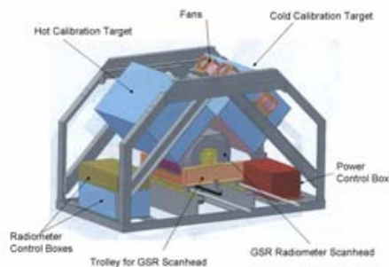
Figure 1. Schematic diagram of the Ground-based Scanning Radiometer (GSR) calibration and scanner system. The GSR scanhead periodically moves out of the framework for atmospheric viewing on a trolley system, and shares time observing the atmosphere and the two thermally controlled blackbody reference targets.
