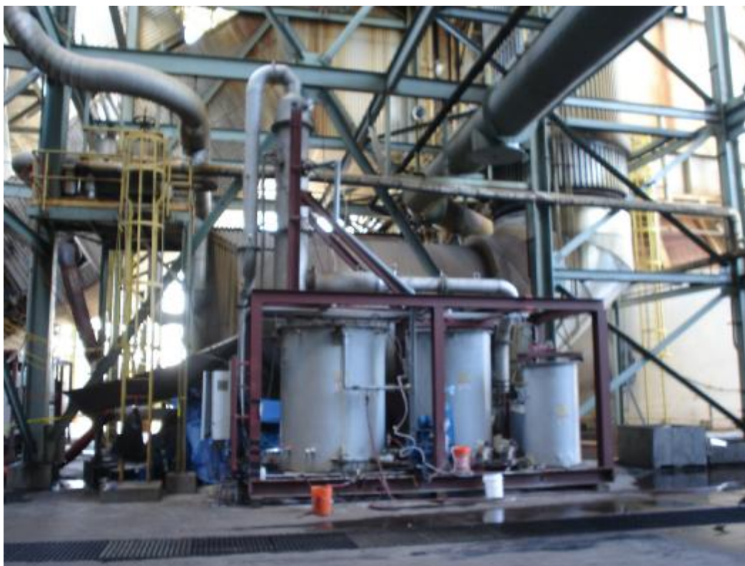
Figure 2. Photo of the Wet FGD Pilot Unit at Monticello Station
