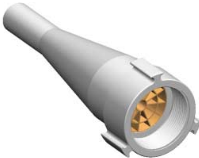
Figure 4.1 Proposed improved sluicing nozzle with integral removable flow straightener and spanner dogs.
