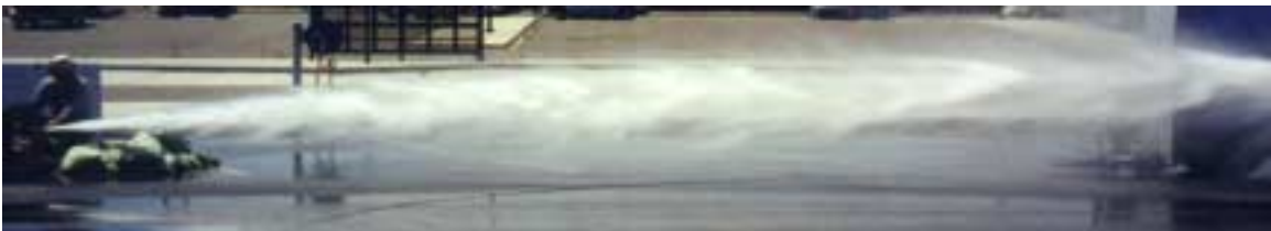
Figure 2.15 Test 30 - Elkhart Nozzle with no flow straightener.
