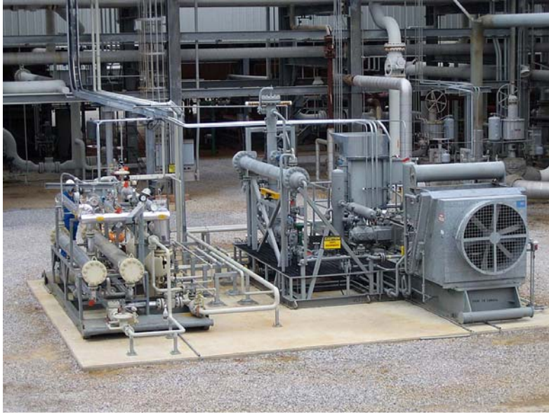
Figure 1. MTR's field demonstration membrane-based gas treating unit at BP Amoco's gas processing plant in Pascagoula, MS. The unit operated virtually continuously from December 2005-September 2006 with essentially constant conditioning performance.
