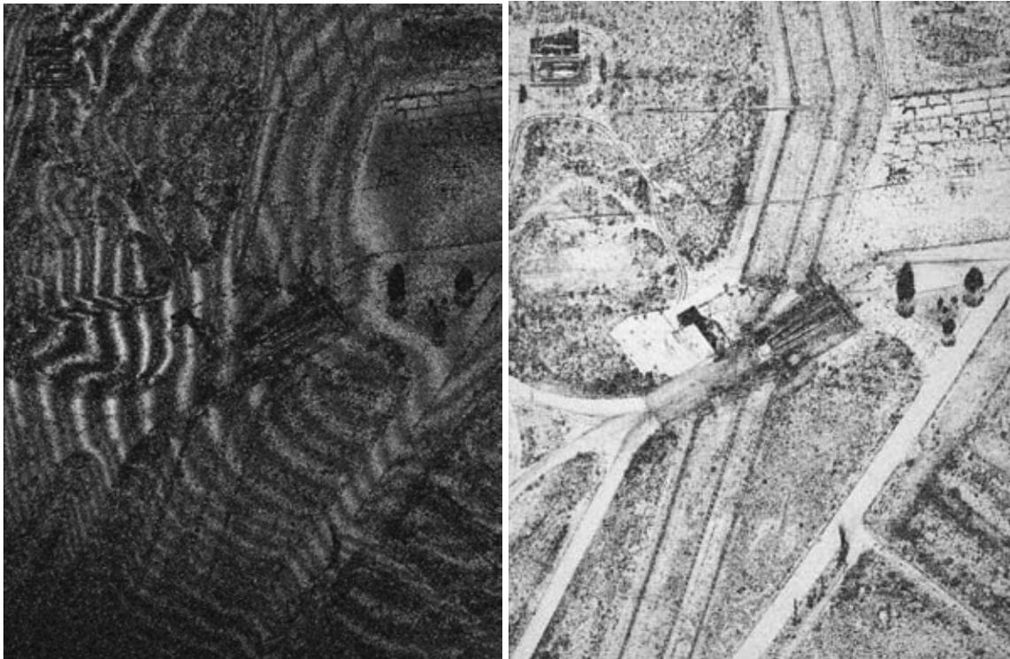
**Figure 4.** The left CCD product was generated from images that were warped with spectrums centered at half the sampling frequency. The right CCD product was generated from images that were warped with spectrums centered at DC.
