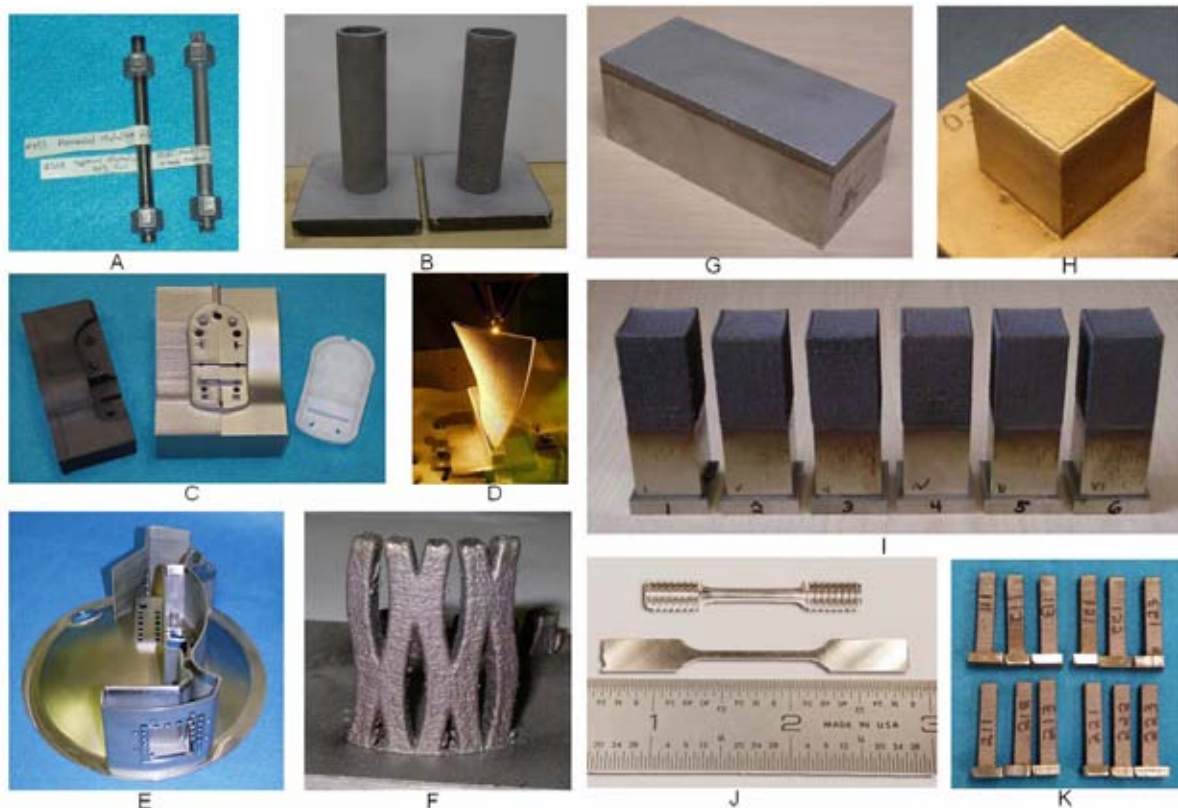
Figure 2.2.A: Examples of Parts Produced by LENS Including Nitinol Lugs (A), 304L Tubes (B), Tool Steel Mold Insert (C), Hollow Turbine Blade (D), 316L Housing (E), and Freeform Optimized Structure Section (F). Also Shown Are Materials Test Samples (G, H, I) and Tensile Samples (J) Machined From LENS Deposited Columns (K)
