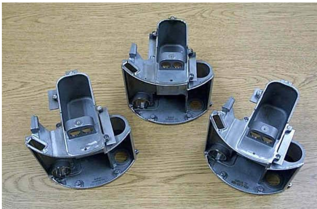
Figure 4.2.1: View of three W87 Firing Set Housings repaired with LENS
