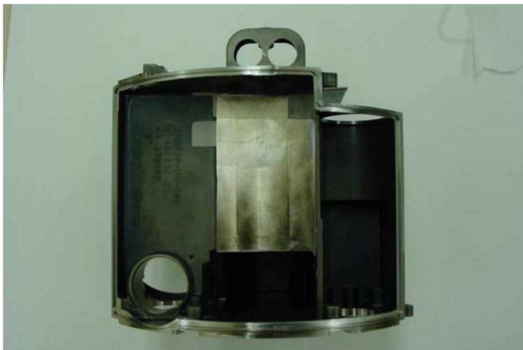
Figure 3.4.1.A: View of Cover Weld Flange after Machining
