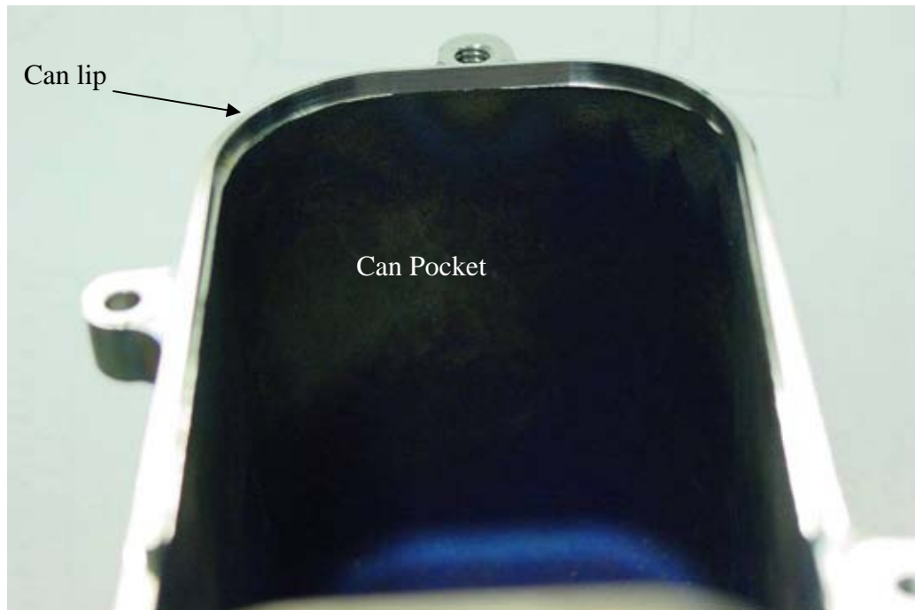
Figure 3.4.1.E: Can lip after machining
