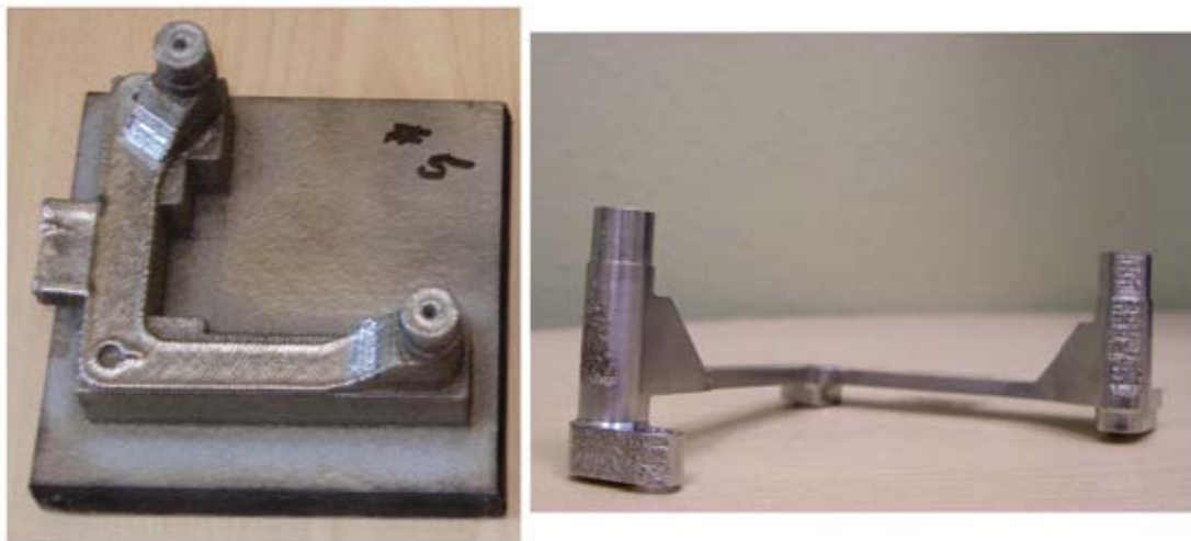
Figure 4.3.2.A: LENS Deposited Brackets in Near Net Shape and Finish Machined Showing Some of the Lessons Learned
