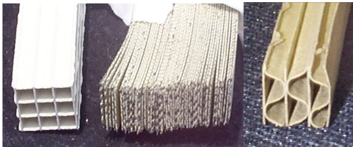
Figure 4. From left to right, honeycomb, plate, and hybrid SCR catalysts.
