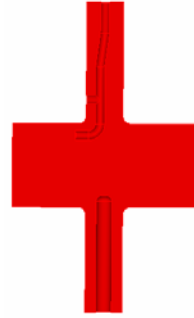
Figure 9: LOM coupler for the ILC crab cavity.
