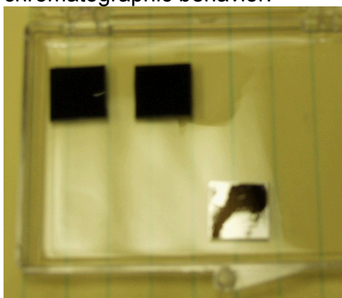
Figure 4. Silicon chips coated with carbon nanotubes. Chip in lower right shows most of the nanotube matrix detached as a result of immersion in water.
