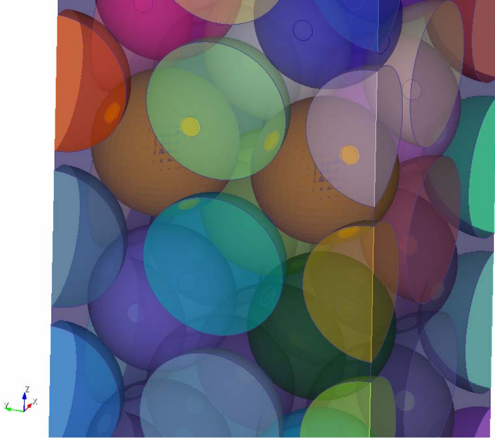
Figure 7. Picture of the filler in the attached phase. Two interior filler particles are highlighted to illustrate the small circles which are the common contact areas between neighboring filler particles.
