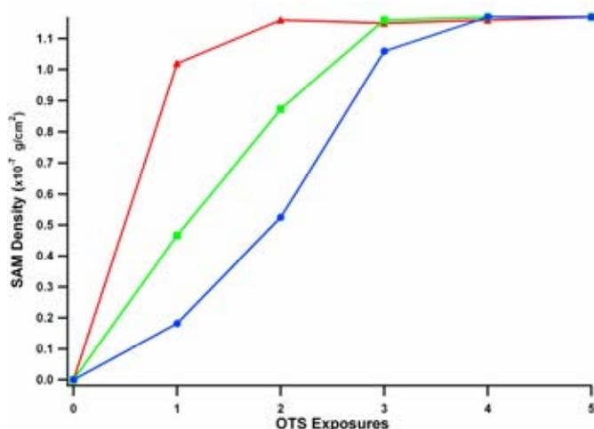
**Figure 2.** Gravimetric C-8 SAM density saturation on microbeads with various diameters, ( $\blacktriangle$ ) 10  $\mu\text{m}$ , ( $\blacksquare$ ) 20  $\mu\text{m}$ , and ( $\bullet$ ) 30  $\mu\text{m}$  (10 nm pores), resulting from increasing numbers of OTS exposures. SAM saturation density is based on a calculated close-packed  $\text{SiC}_8$  density of  $1.17 \times 10^{-7} \text{ g/cm}^2$ .<sup>46</sup>
