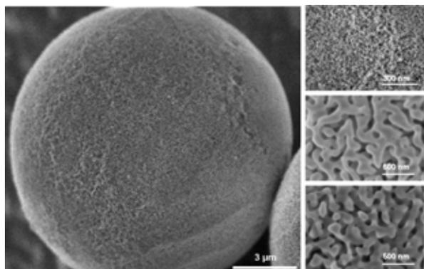
**Figure 1.** SEM images of silica microspheres with varying surface structure. Left: 10,000 $\times$  image of a 10  $\mu\text{m}$  bead with 10 nm pores. Right, descending vertically: 200,000 $\times$  images of beads with 10 nm pores and 100,000 $\times$  images of beads with 50 and 100 nm pores.
