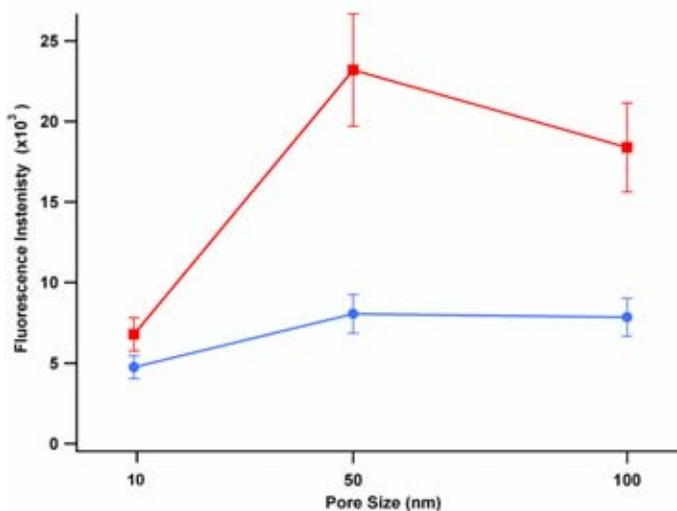
**Figure 4.** Relative surface areas of (■) EPC and (●) DPPC (each with 0.5% mol/mol Rhodamine DHPE) bilayers on 10 μm beads with varying pore structure. Fluorescence intensities are corrected for the EPC fluid-phase head group area versus the DPPC gel-phase head group area.
