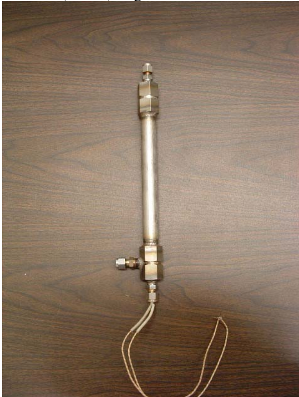
Figure 2: Air heater for air supply subsystem
