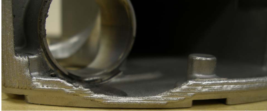
Figure 18. This Cover Flange Weld Lip Feature Presented Problems Due to No Existing Material On Which To Build the LENS Weld Flange. This Would Be Easier with 5 Axis Depositing or a Different Fixture.
