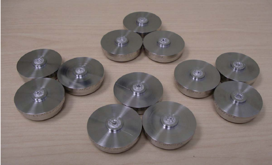
Figure 4. The Full Set of Repaired Weld Bases with Bore Diameters Oversized by (CW from Left) 0.015", 0.030", 0.045", and 0.000"(Nominal)
