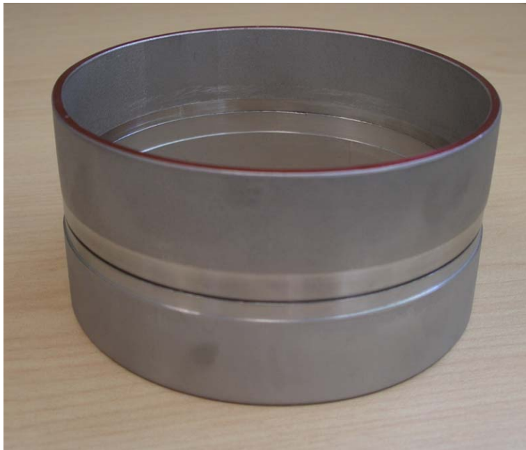
Figure 14. The Assembled Step Joint Rings
