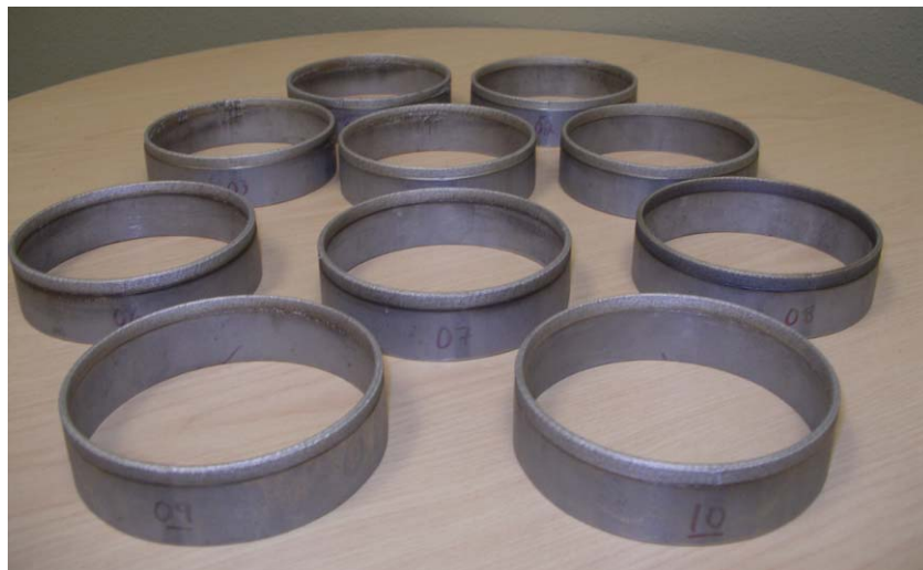
Figure 10. The Full Set of LENS Repaired Step Joint Rings
