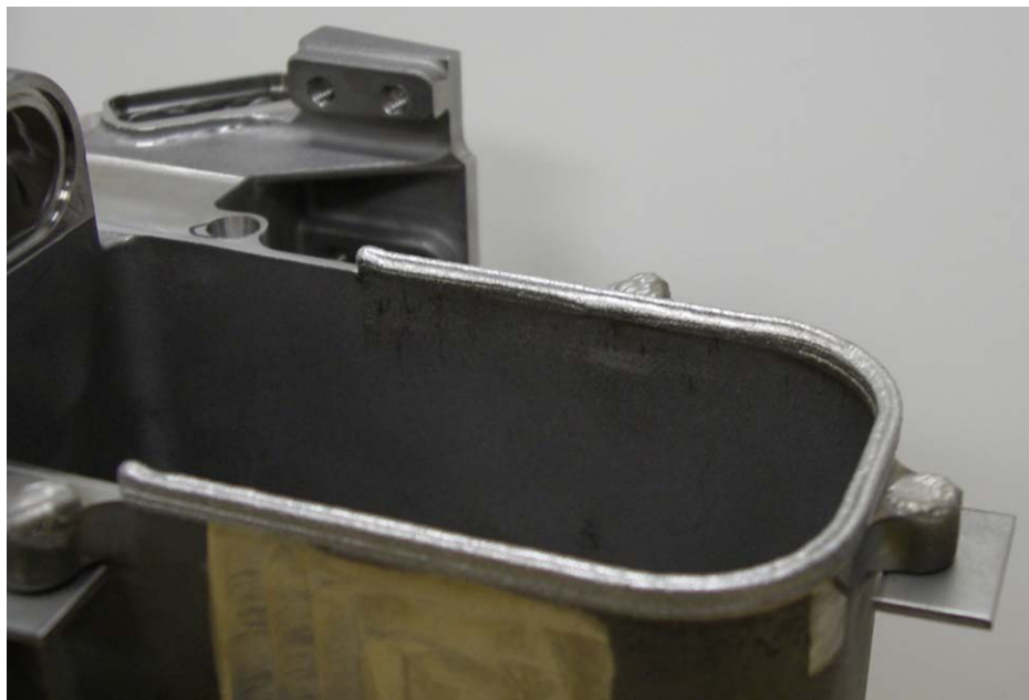
Figure 21. The Completed Can Lip and Filled Bolt Holes. Note the Large Feature on the Far Left Prevented the Entire Can Lip from Being Completed. Also Note the Support Plate Used Under Each Hole to Help the LENS Build Start
