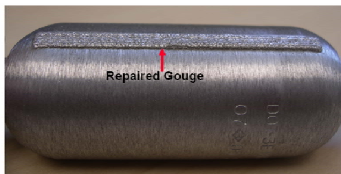
Figure 9. Repaired Gouge in Sample Gas Bottle
