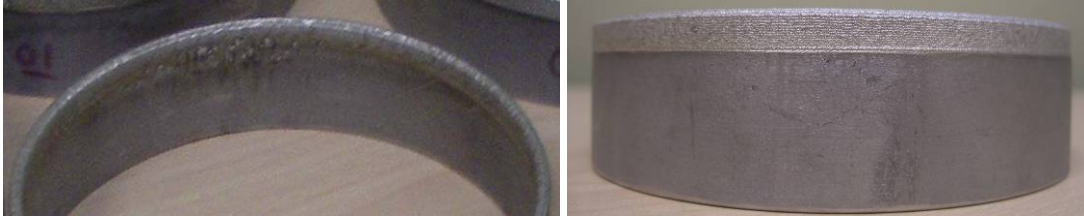
Figure 12. Some Rings Were Not Very Round Causing The Laser To Fall Down the Side of the Bore Leaving Spatter (Left) with a Round Ring for Comparison (Right)
