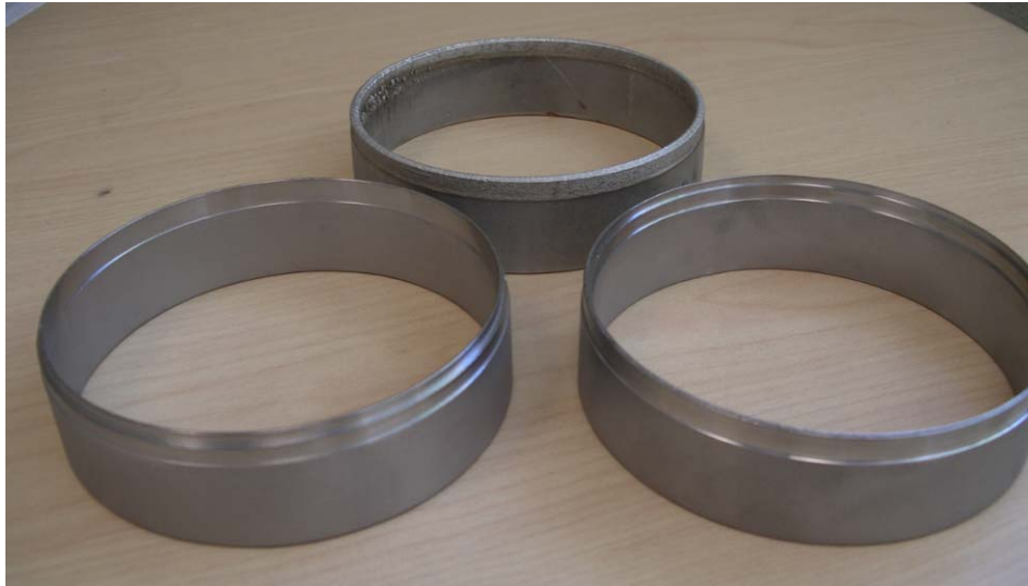
Figure 13. Two Rings with the Step Joint Machined Into the LENS Material with a Net Shape LENS Ring Shown for Comparison
