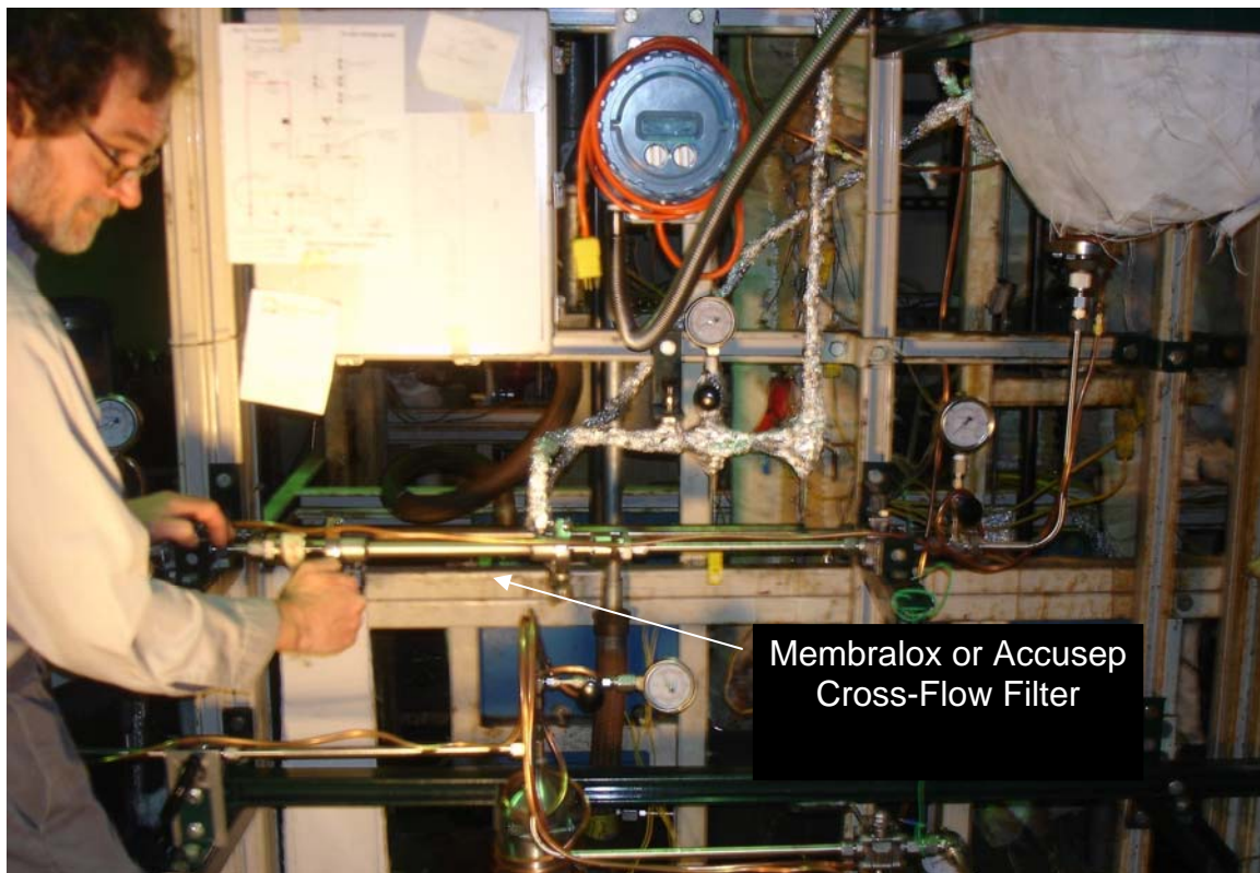
Figure 6. Installation of the Filter Tube Assembly.
