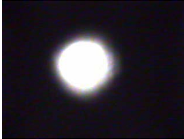
Figure 6: Image of the IR beam in the probe when reflected by a plane mirror.
