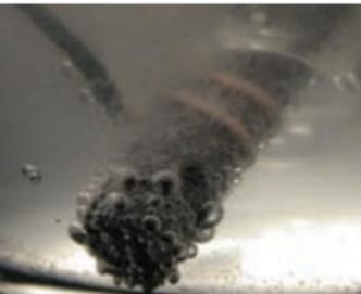
▲ Hydrogen production – via off-peak electrolysis
