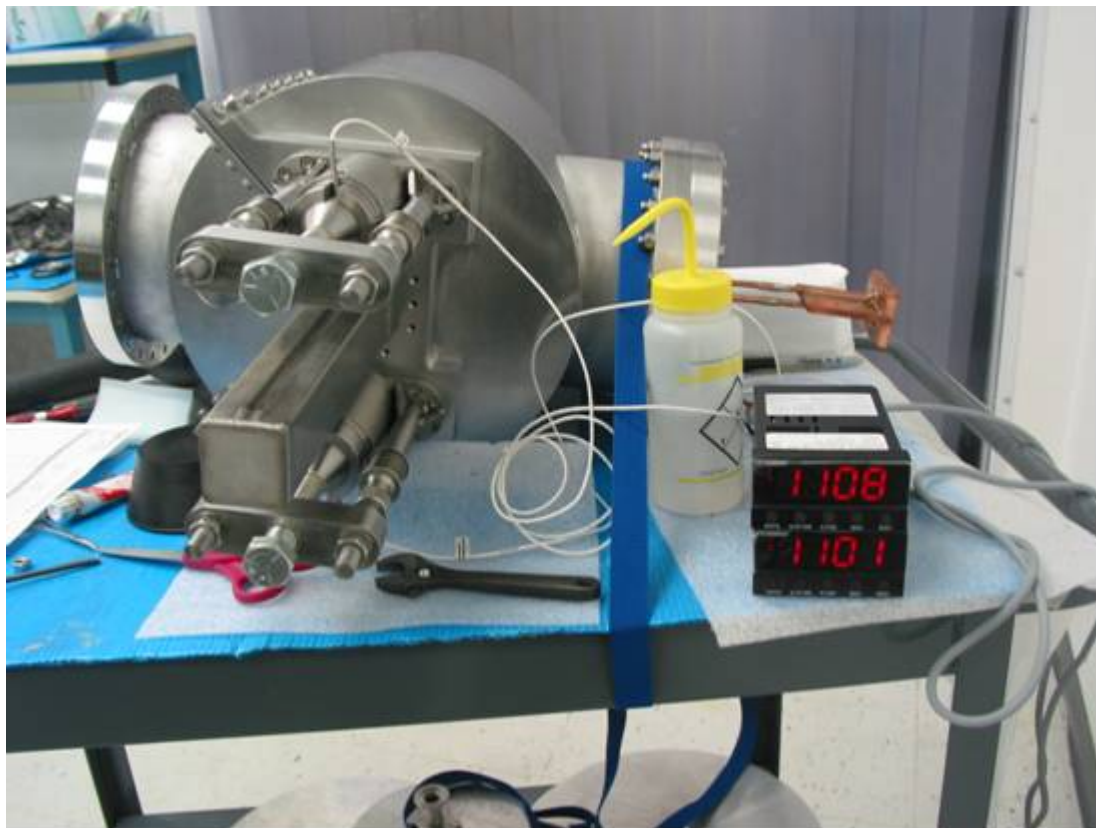
Fig. 16. Loading test, force on the interfaces is 2.2 tones, about 22 kN.
