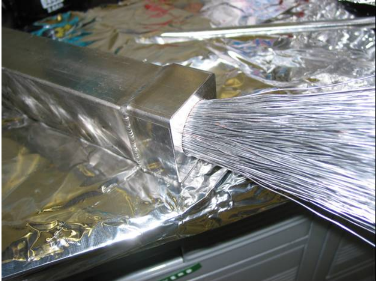
Fig. 6. Transition piece welded to the CS2 conductor.
