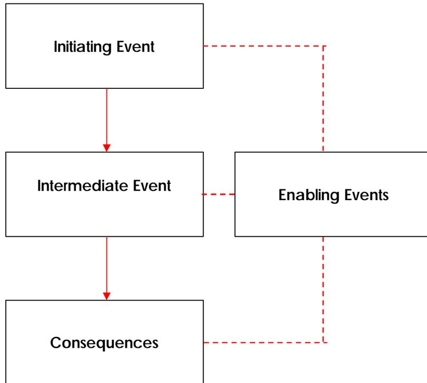
**Initiating Event:** The cause (component failure – operational mistakes – external occurrence).
