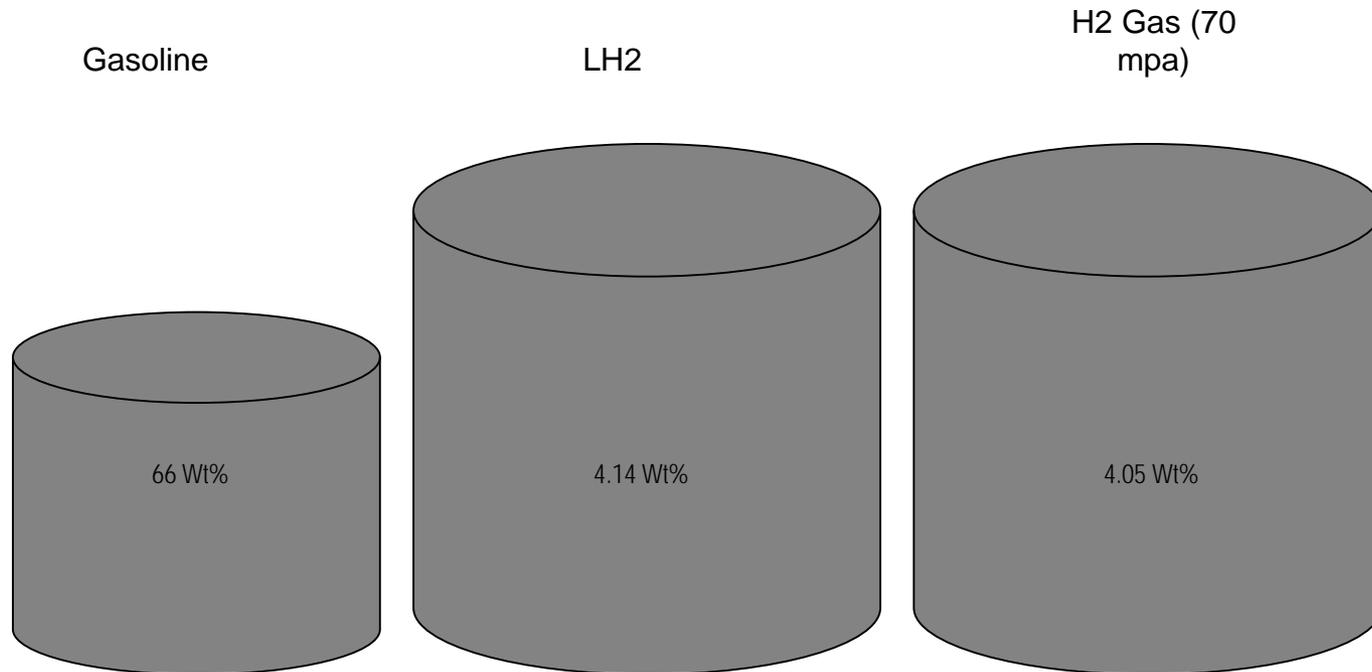
*Calculation of the gravimetric energy density of fuel needed to drive 250 miles.
