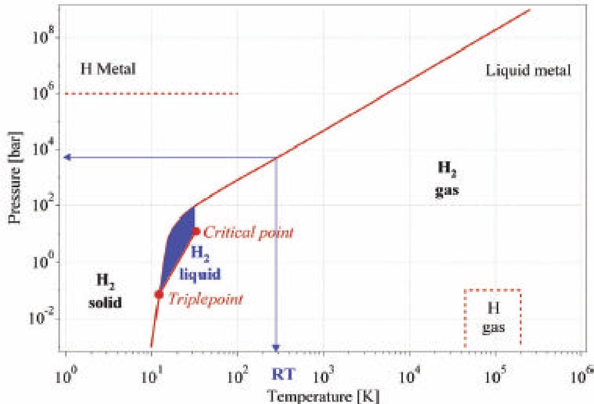
*Liquid hydrogen only exists between the solid line and the line from the triple point at 21.2 K and the critical point at 32 K.*
