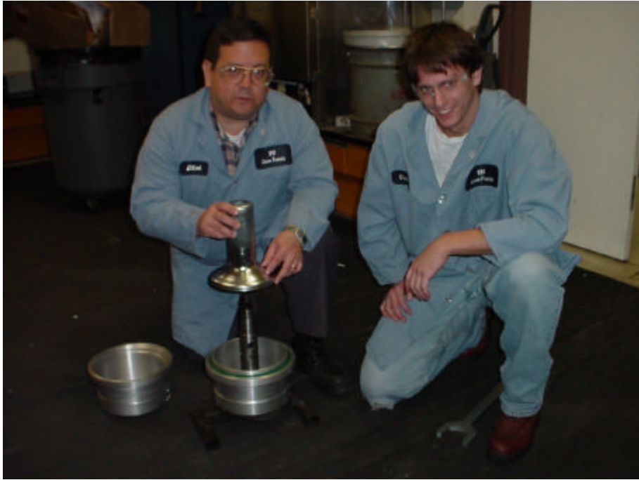
Figure 12. Spinner-II Model 600 Centrifuge Assembly.
