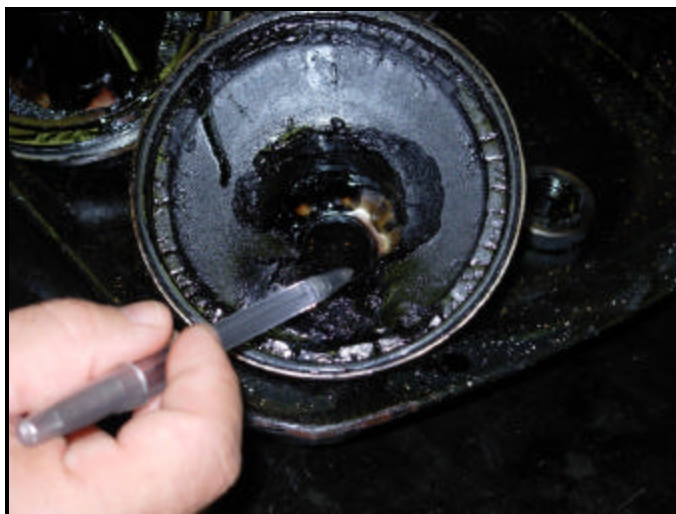
Figure 10. The Cover Removed from the Spinner II Model 60, showing the solid “Cake.”
