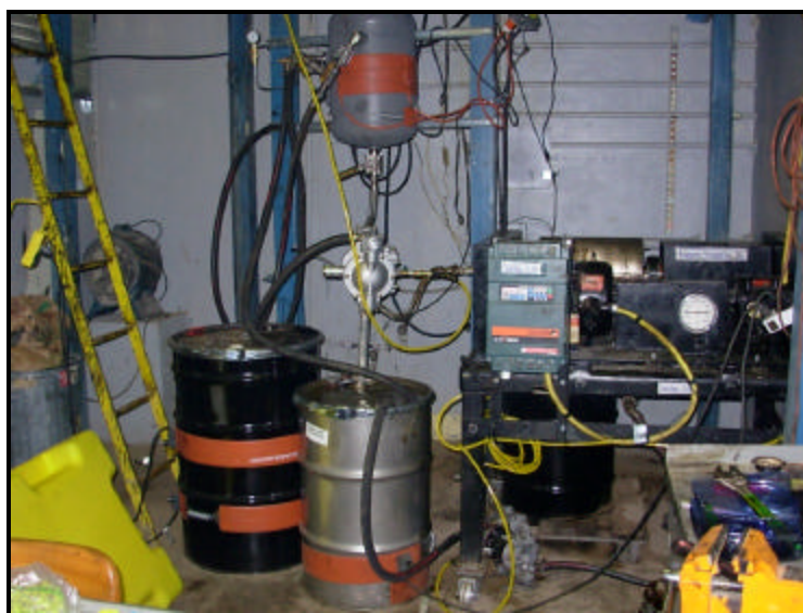
Figure 2. Installation of the Sharples Pennwalt Decanter-Type Centrifuge.
