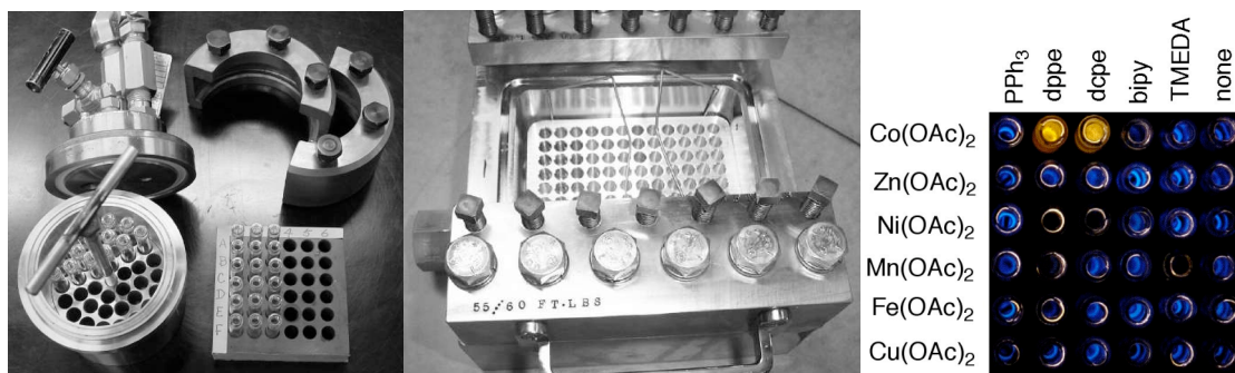
Figure 1. High-pressure vessels for combinatorial testing of catalysts, capable of testing a 6x6 array at 200 bar (left) and an 8x12 array at 100 bar (centre). The colorimetric assay method is illustrated at right, where catalytically active metal/ligand combinations appear yellow while inactive combinations appear blue.
