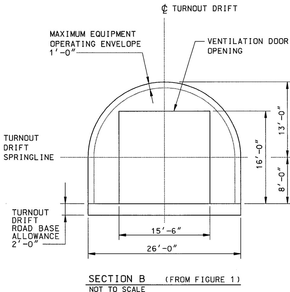
Figure 3. Turnout Drift Ventilation Door Elevation View
