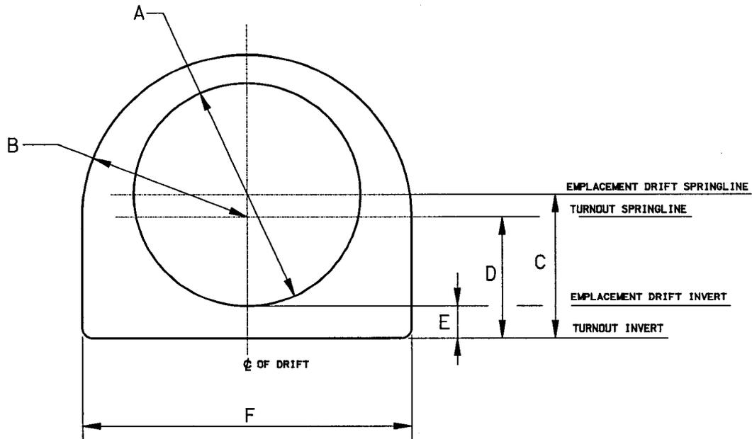
Figure 2. Turnout Drift and Emplacement Drift Interface View
