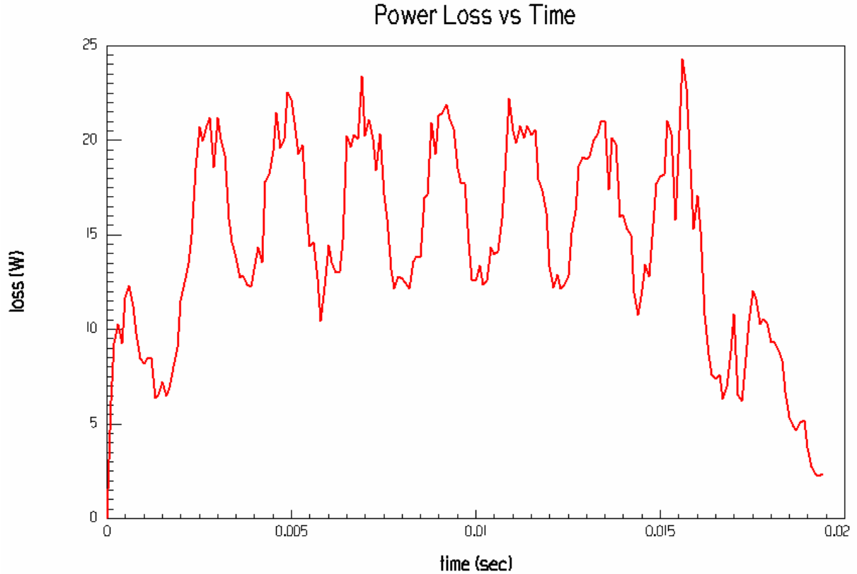
Figure 42 Eddy-current power loss for a notched experimental Ti6Al4V wheel at 600 rpm.
