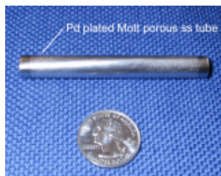
Figure 4. Pd membrane deposited on the outside of a Mott 0.1 \mu\text{m} grade symmetric stainless steel support tube.
