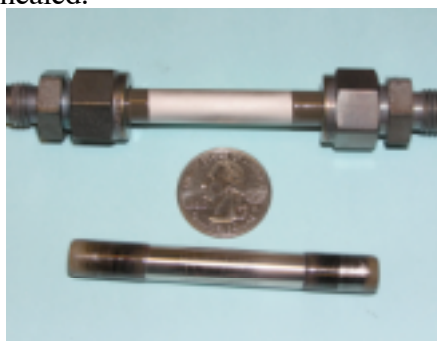
Figure 1. Pd alloy membranes deposited on the outside of GTC-200 symmetric supports. The coin has a diameter of 2.4 cm.
