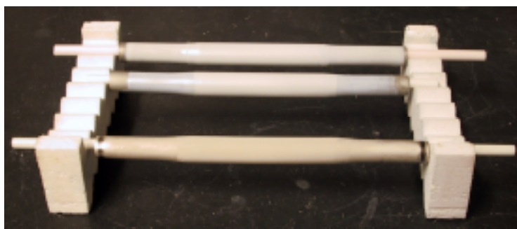
Figure 3. Two Pall AccuSep \text{ZrO}_2 coated porous stainless steel filters at top. Pd coated AccuSep filter at bottom. These substrates have approximately 30 \text{cm}^2 of active area.
