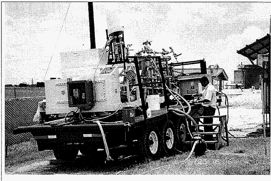
Figure 2 shows the GPRI desalination trailer during its trial run.
