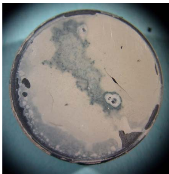
Figure 20. Delaminated AlN film on Hexoloy SG substrate after heating.
