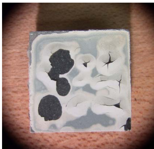
Figure 14. AlN film on siliconized SiC after 700°C thermal cycle.
