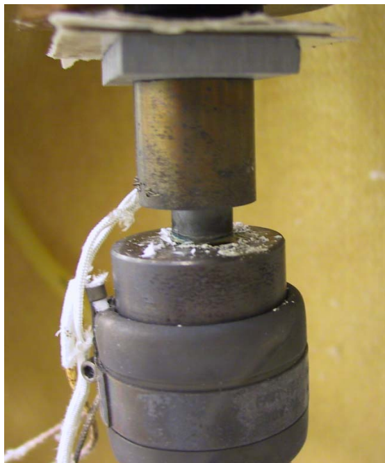
Figure 49. Glass couplant test setup prior to heating.
