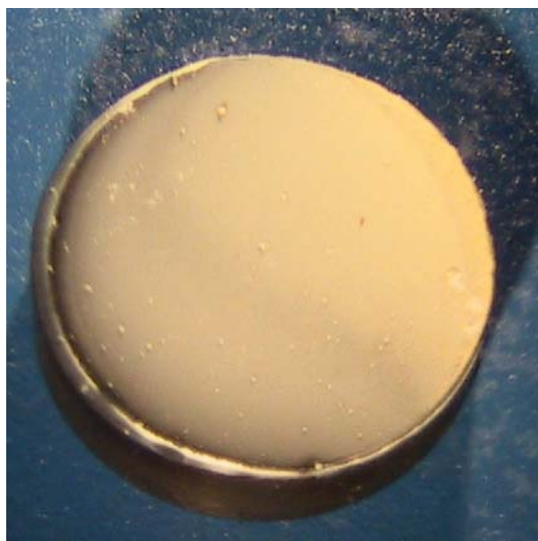
Figure 10. As-deposited AlN film on conductive bulk AlN substrate.
