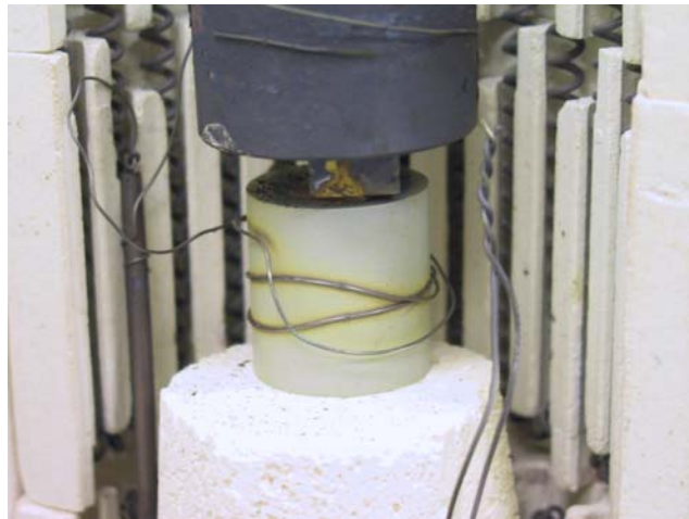
Figure 31. Simulated transducer in furnace after test.
