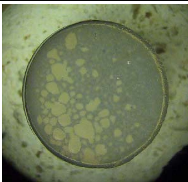
Figure 16. AlN film on porous SiC cylinder after 200°C thermal cycle.
