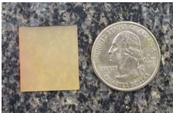
Figure 27. LGS crystal, as received.
