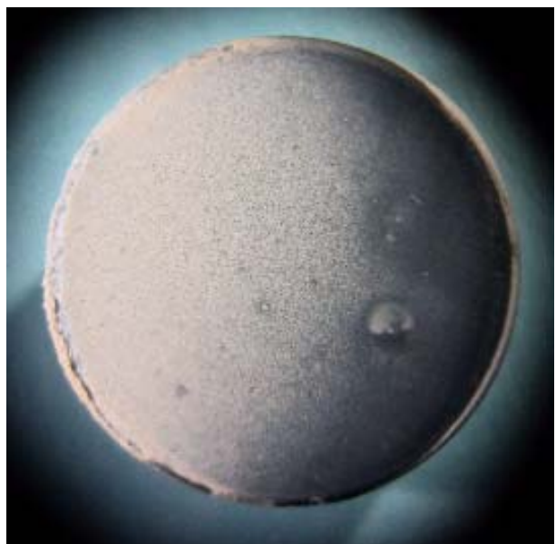
Figure 8. As-deposited AlN film on Performance SiC .
