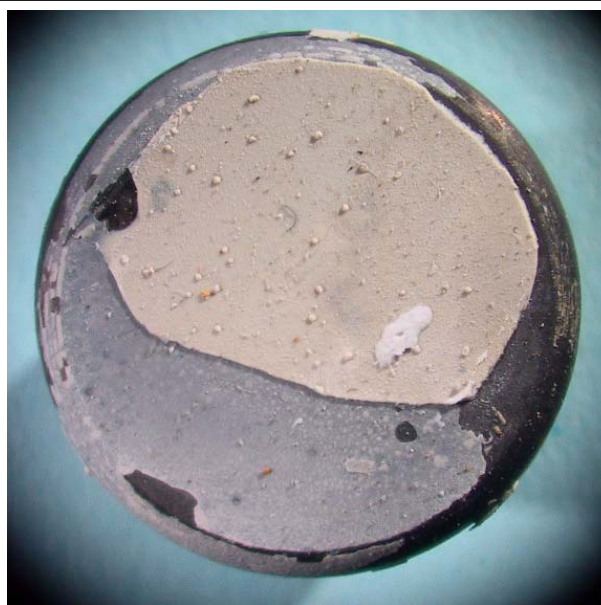
Figure 17. AlN film on Ti delaminated by heating.
