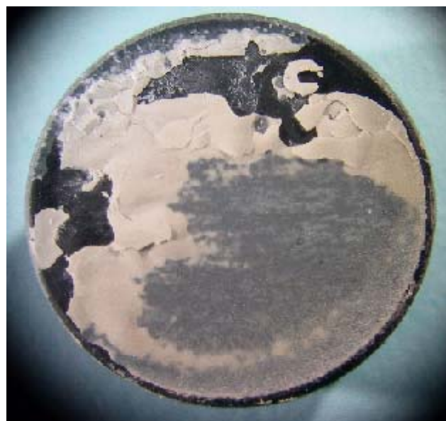
Figure 19. Polish-damaged AlN film on Performance SiC substrate.
