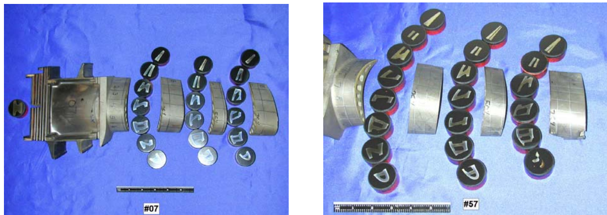
Figure 7-2: Photographs showing metallurgical sample locations in Blade 7 and 57
