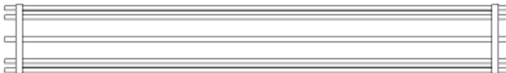
Line drawing of the 45 L accumulator body. The body is of carbon fiber composite. Dimensions are 79.5" long, 11" diameter.
