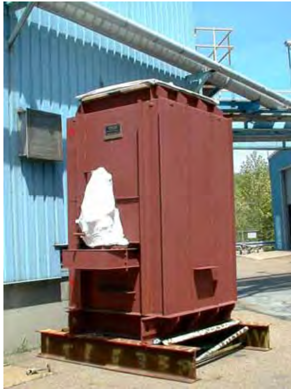
Photo 3-B. Ljungstrom-Type Pilot Air Heater (Before Installation)
