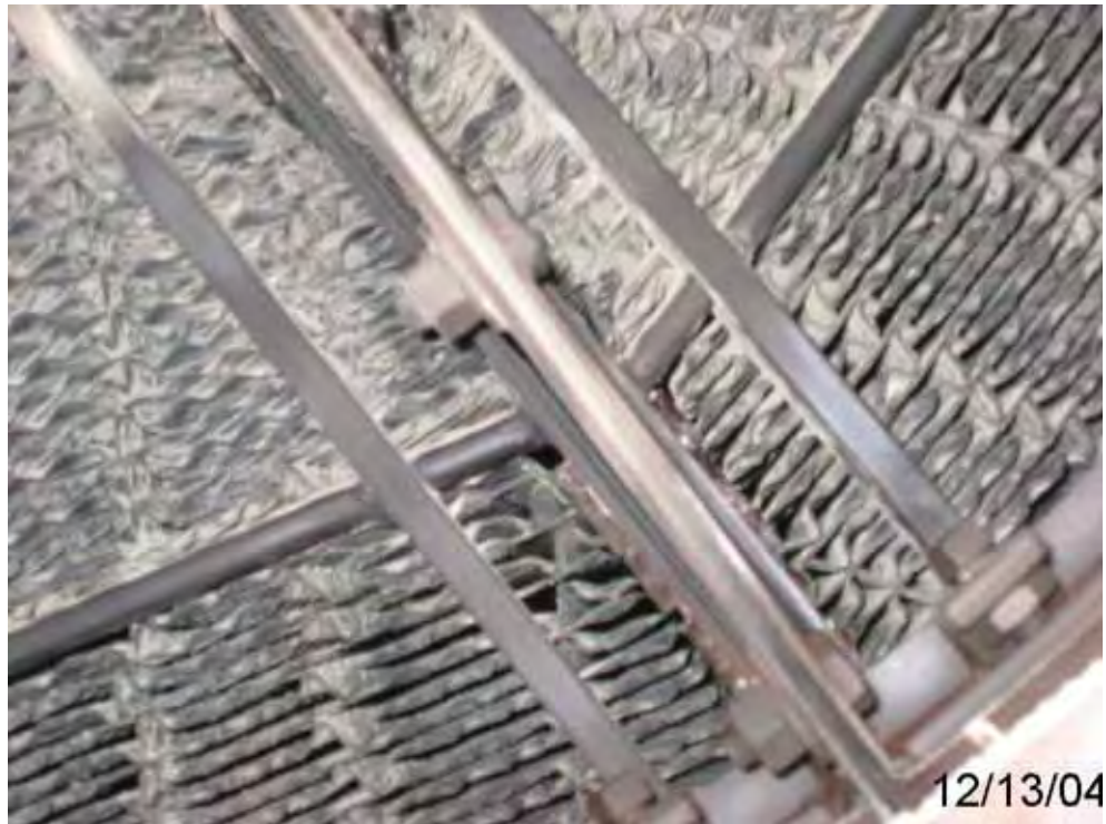
Figure 40. Cold End Basket Before Soot Blowing
