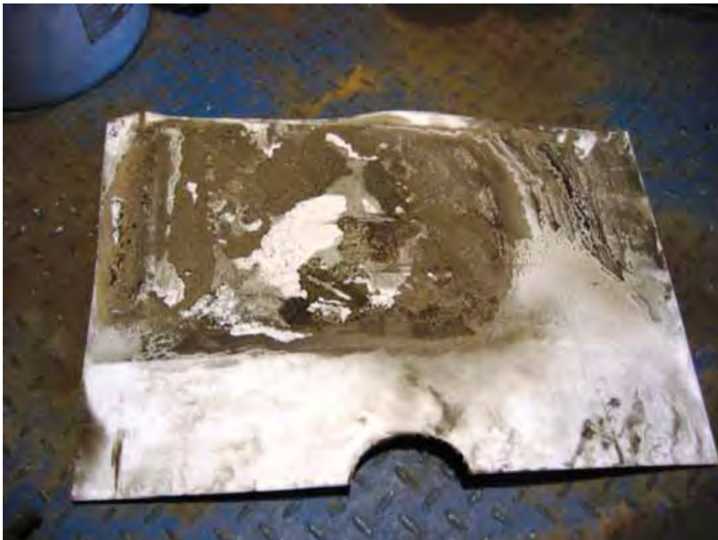
Figure 17. High Carbon Fly Ash Accumulation on Pilot ESP Teflon Barrier, Field #1
