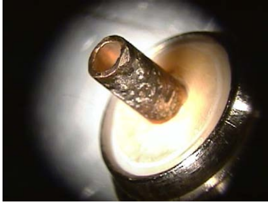
Figure 18: High voltage electrode following insulation material testing.
