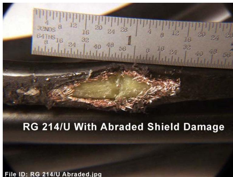
Figure 3: Abrasion on coaxial cable
