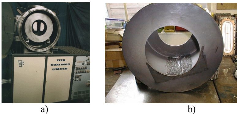
Figure 2- a) Picture of the barrel coating system b) Close-up picture of the barrel with some material inside (not our microspheres)
