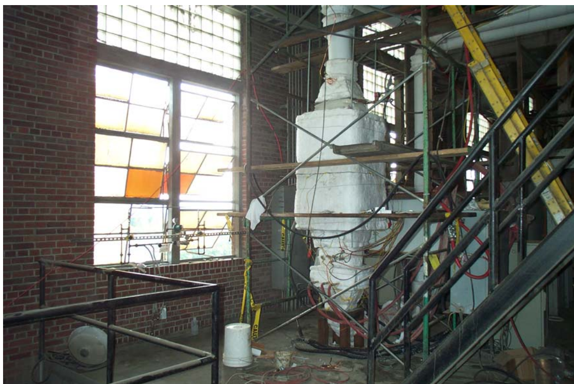
Figure 9. Slipstream reactor after insulation.
